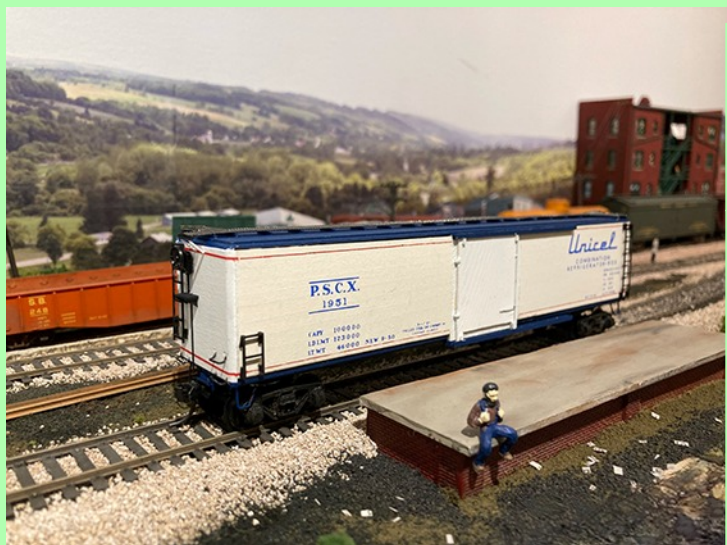
Ed O'Rourke – edwardorourke1@me.com – HO scale – Ambroid Unicel refrigerator car. Produced by Pressed Steel Car Co, it was built out of plywood. They were lightweight and well insulated so they held the cold well without icing. The ARA did not accept them for interchange service, so the project died.
