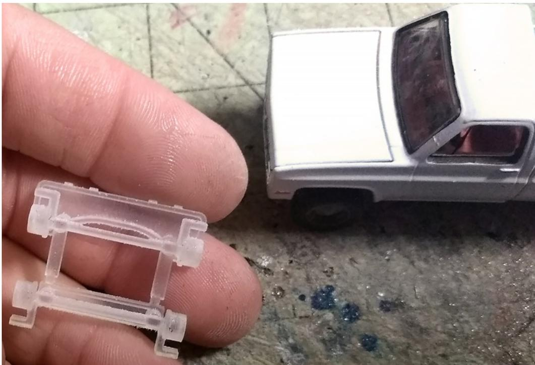
The first step I do to use these or any 3D printed components was to separate the parts far enough to be able to clean thoroughly with a tooth brush and rubbing alcohol.
