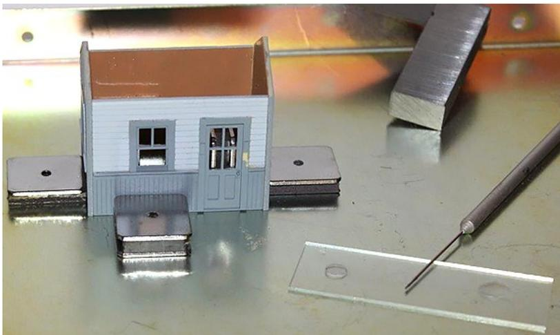
*I used a jig purchased from Micro Mark to assemble the house one corner at a time. You can see the tool I used to apply glue, along with the machinist square I used to keep everything square.*
