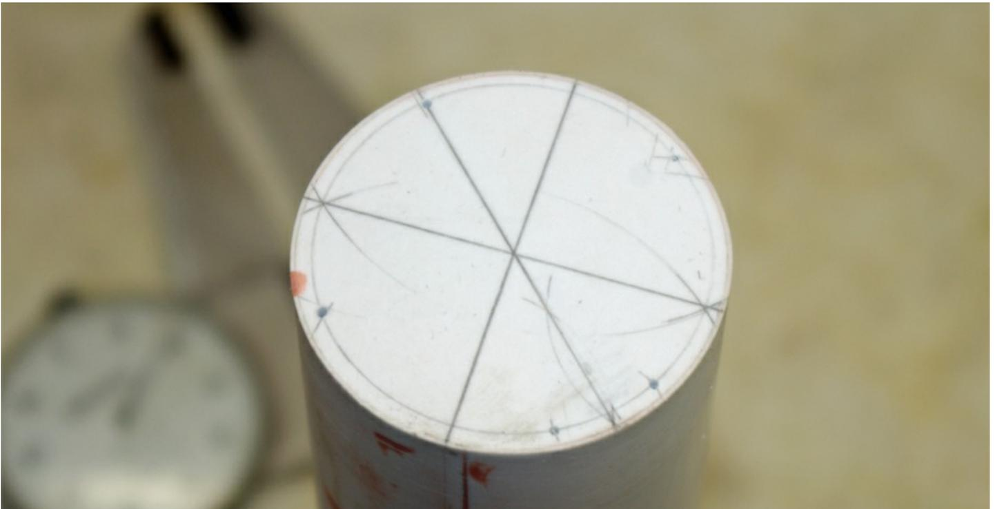
*Here is the top of one of the tanks showing the holes for the railing posts. I drilled the single post hole at the top left first and then the two at the lower right. Next, I set the compass to about half way and scribed two marks to help locate the other two railing post holes. Look closely and you will see the compass lines near those holes.*
