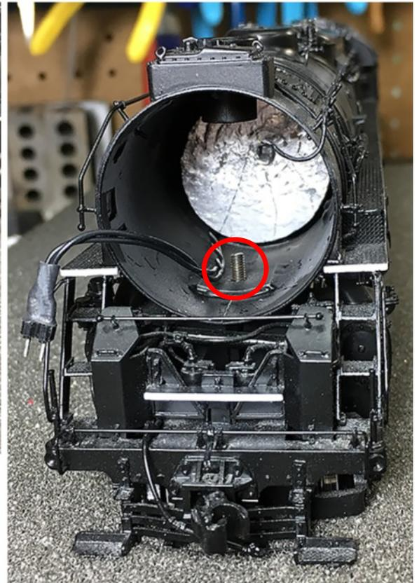
*ABOVE RIGHT: The boiler screw is circled in red. More on that on the next page. After seeing the size and placement of the weight, I determined that using the boiler for the decoder would not work. There was, however, plenty of room for a round high bass speaker.*
