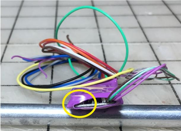
*CurrentKeeper plug was covered on the left side of the decoder.*
