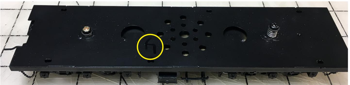
*We got lucky here. Normally, in older tenders you have to drill holes for the speaker. This has a subfloor and the ends of the tender are open, thus allowing the sound to go through the holes and out the ends. The small arrow I drew (see yellow circle) shows me how far back I need to stay with the install for height.*
