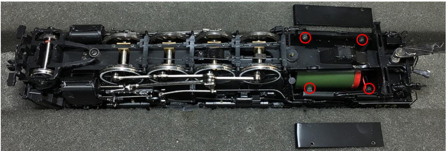
*Ash pan covers removed. Note that I replaced the screws back into their holes so I didn't lose them.*
