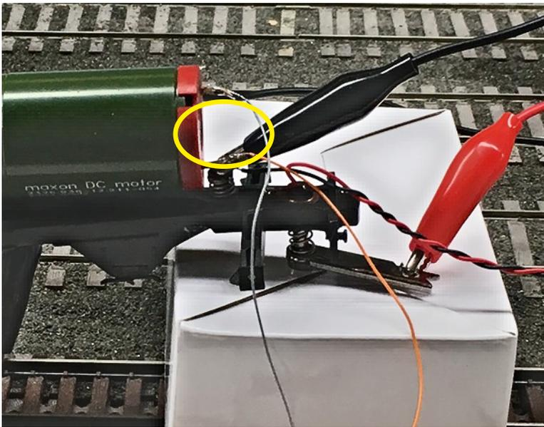
At one point in testing set up, both LED's started blinking and the locomotive stopped running. That's not good. What had happened was the black clip going from the track to the locomotive frame accidentally touched the motor lead, causing the motor to no longer be isolated, and the decoder went into an error. No damage was done, but it's worth noting, and knowing what specific decoder error codes mean.
