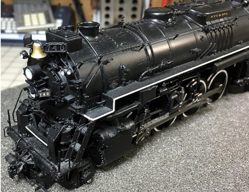
*LEFT: To begin disassembly of the locomotive, I started with the smoke box door. In most cases, this is a press fit where you can very carefully pull it out of the smoke box. (I have an O Scale locomotive that used two extremely small screws to hold the door to the smoke box so check that on your models before trying to remove.) Go slow and watch for any other piping that may have to be removed first. This locomotive had a press fit that was relatively easy to remove.*
