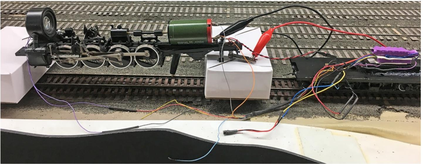
*For this test, the 2x3 mini connector on the locomotive side is used, but the wiring is just temporary on the locomotive. Notice that the red and black clips from the track power to the model frame and drawbar are being used because we are not sitting on the track.*
