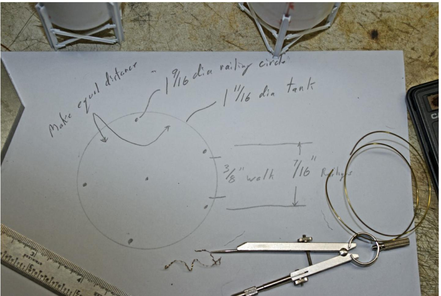
*I made a sketch again to determine where to drill the holes for the posts in the top of the tanks. You can see I have also pre-bent some wire for the railings. I bent this around a piece of tube, and will cut it to length later.*
