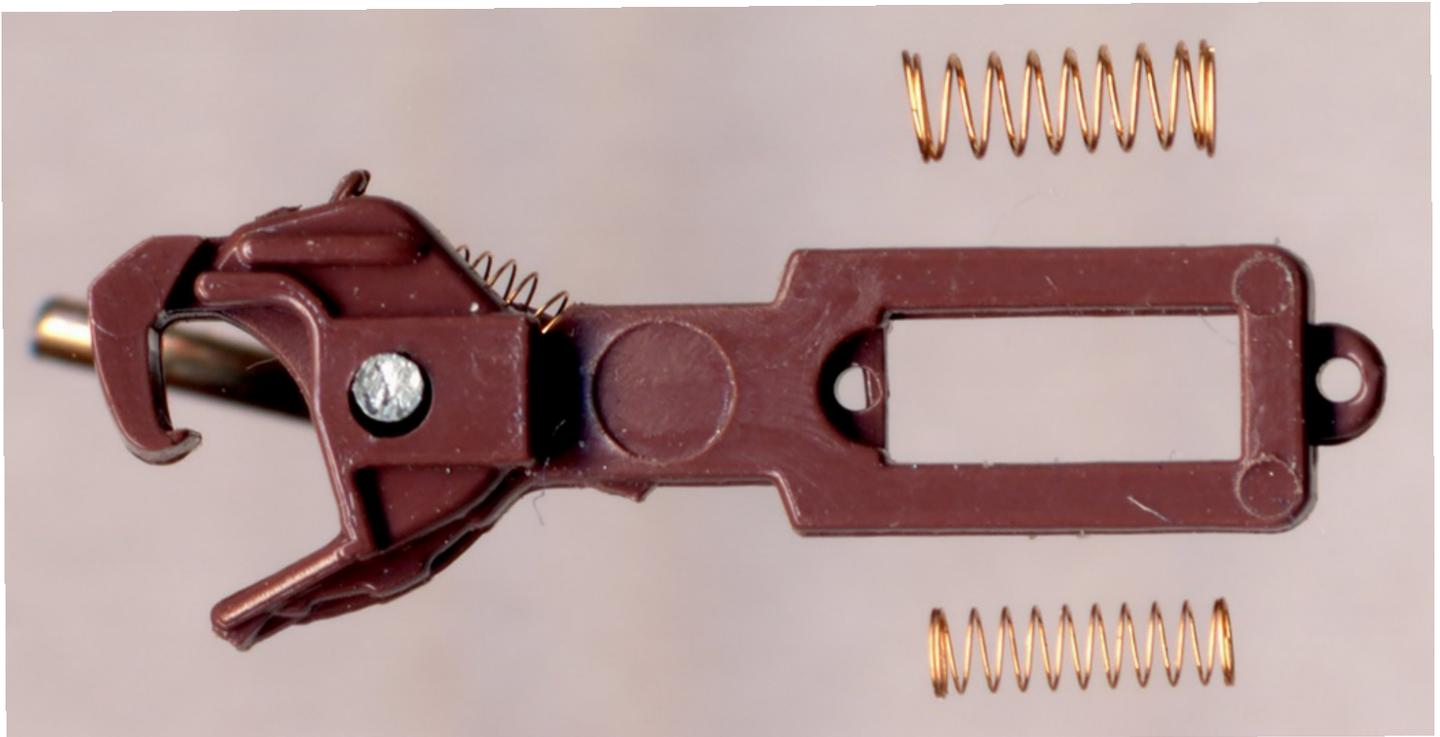
*A Kadee No. 808 poses between the standard centering spring (top) and a No. 817 knuckle spring (bottom). Both springs are the same length, but the knuckle spring has more coils and a smaller wire diameter. The knuckle spring’s smaller wire diameter makes it 80 percent softer than the centering spring. The fact that it has ten coils, as opposed to the centering spring’s eight, reduces its stiffness by another 20 percent. The total reduction amounts to about 84 percent. Author’s photo.*
