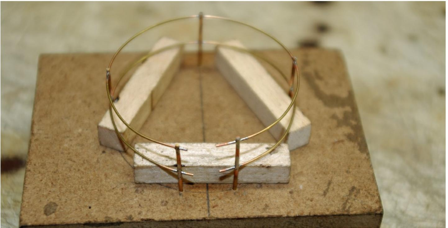
*This is the fixture I came up with. It worked, but the railing wire was still too stiff and hard to bend to the right curve. It was so stiff that it would pull the posts out of square as you can see in the photo. I was getting close, but I wasn't there yet, so I kept trying.*
