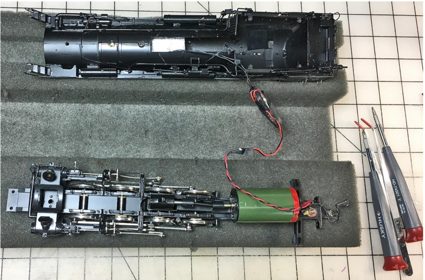
Putting the locomotive aside, I looked at the decoder and bench tested it. First, I had to remove the shrink wrap covering the plug in of the CurrentKeeper (see yellow circle below). An X-ACTO took care of that.
