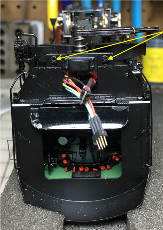
*LEFT: I had forgotten to take a picture of the rear cab screws that needed removing, so this was shot after the install.*
