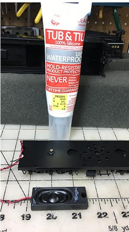
*Using pure silicone, spread some on the ends of the speaker enclosure and place the speaker on the deck of the tender. Next, put silicone around the speaker to seal it to the deck. While not very pretty, it will stop any movement of the enclosure (vibration). In addition, it will allow this to be removed someday, if need be, without causing any damage to the deck.*
