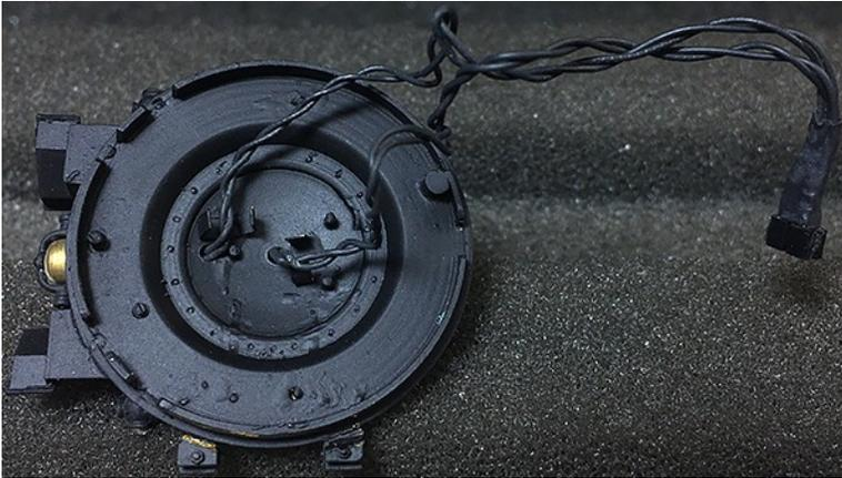
Original wiring on left. Two bulbs wired into one plug. Note the bent over tabs for holding the wires.
