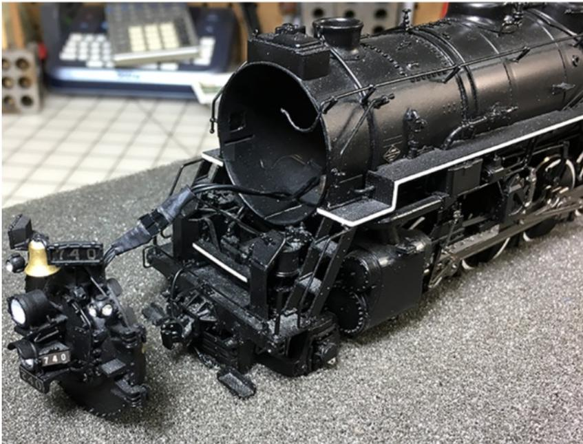
*ABOVE: Smoke box door removed. Note the wiring and plug for the front headlight. In this case, the piping did not need to be removed as we could work around it.*
