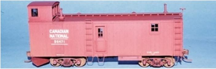
This kit includes the special diamond flanger blade, stirrup steps, wind deflectors for the cupola, brake cylinders and handbrake wheels, and a choice of smoke jacks for coal or oil fired stoves (H shape for oil). Extras of the stirrup steps and brake wheels are included. [Check out their Shapeways shop.](#)
