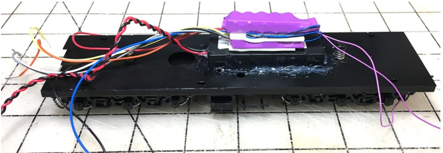
*Using double sided thick carpet tape, I added the decoder and then the CurrentKeeper. I am not worried about any heat built up as it's a 2 amp decoder, and this locomotive will not pull anything over 1 amp. Plus, there is plenty of air around the install.*
