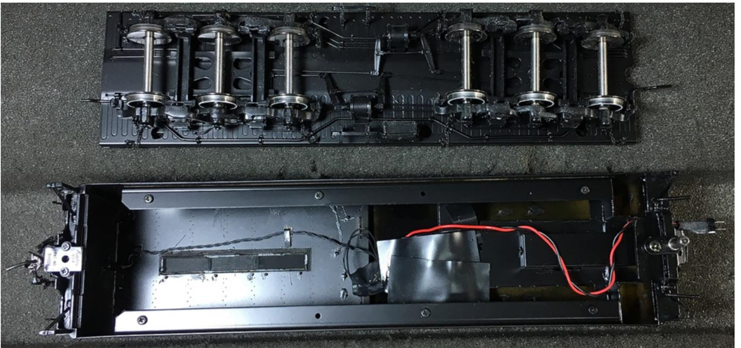
*With the screws safely back where they belong, we can see the plug that went to the locomotive for the rear light. This will be removed as John wants an LED in the rear.*
