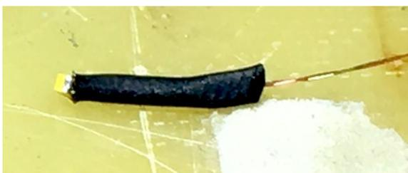
With the LED secured in shrink tube (above), we can glue it into the casting with Canopy Glue Formula 560. It dries clear and stays flexible. On the right, I have a larger piece of shrink tube that will go over the rear light casting and hold everything in place.
