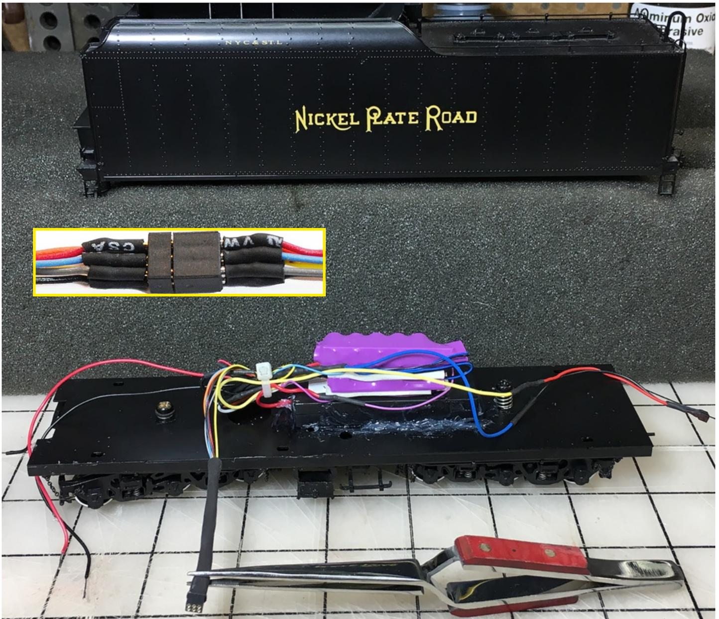
*Two plugs to the locomotive. The red and black wires above will carry track power from locomotive, while the other wires from the decoder will use the 2x3 mini connector. There are other ways of doing this, but not being my engine, I did not want to drill, tap or otherwise do anything to alter the locomotive. I could have taken track power from the tender, but it would have still needed the plug for the locomotive track power.*
