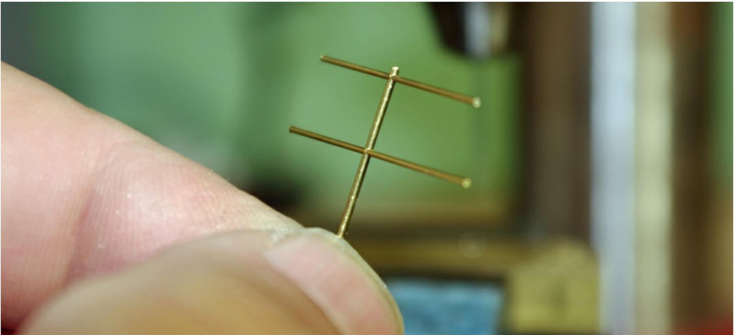
*This is what you should get. Two holes that are parallel and through the post wire. This worked very well, as shown here, but I had some problems later on. When trying to make a curved railing there was just too much handling and the posts would break at the holes. More on that later.*
