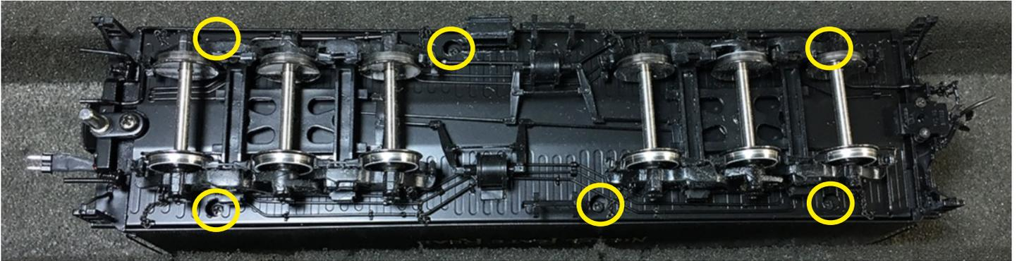
*Six screws hold the tender shell to the bottom. Remove those, and then with the shell off, replace the screws back so you don't lose them.*
