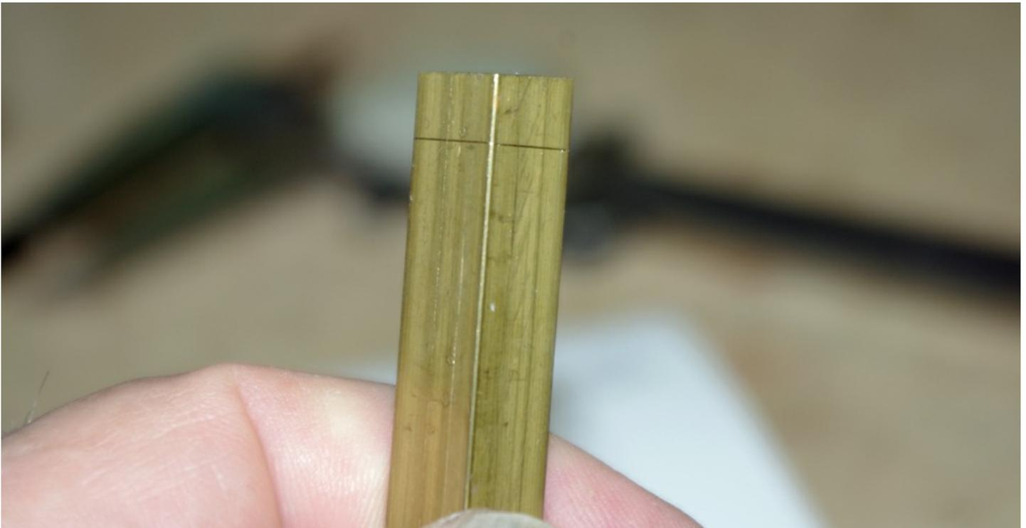
*In this photo, I have scribed my two layout lines. These must be accurate and meet at an edge. On one line, I will drill a hole for the railing post. On the other line, I will drill the two holes for the railings.*
