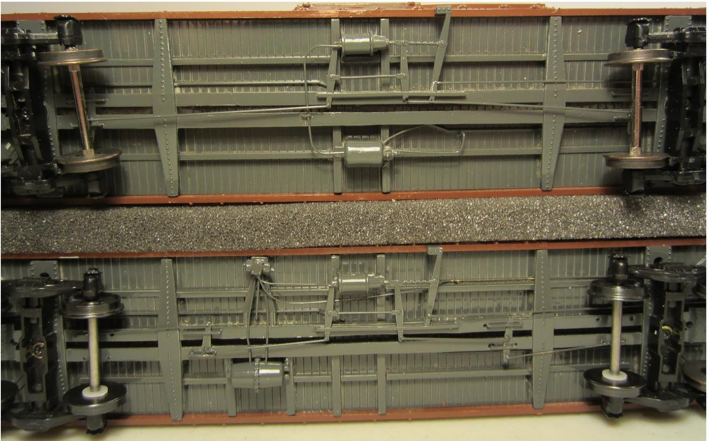
*One other differentiation I made between the PRR X-29 and the NYC Lot 504-B models was in their brake systems. The X-29 is on the top in this photo and has the KD brake system that was supplied with the kit. On the bottom is the NYC car set up with an AB brake system.*
