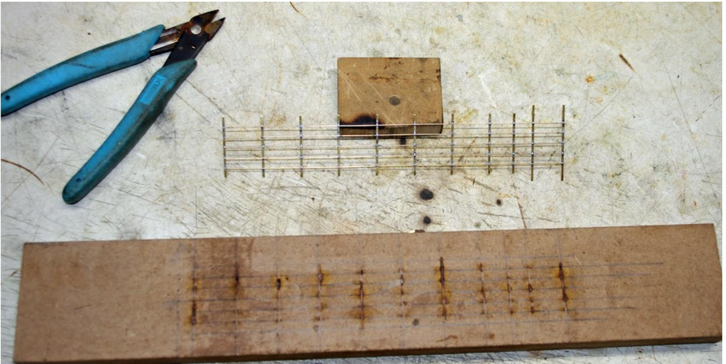
*Here was my first attempt at the ladder cage. Not bad, but I thought the wire was a bit too heavy. Notice I do not have the “feet” on the flat bars bent to solder to the ladder. After I bent this one, and then decided to bend the feet, I realized I had worked myself into a corner. There was no way to get a pliers into the flat bar to bend it, and the chance of them all being bent the same was slim. I needed to try this again.*
