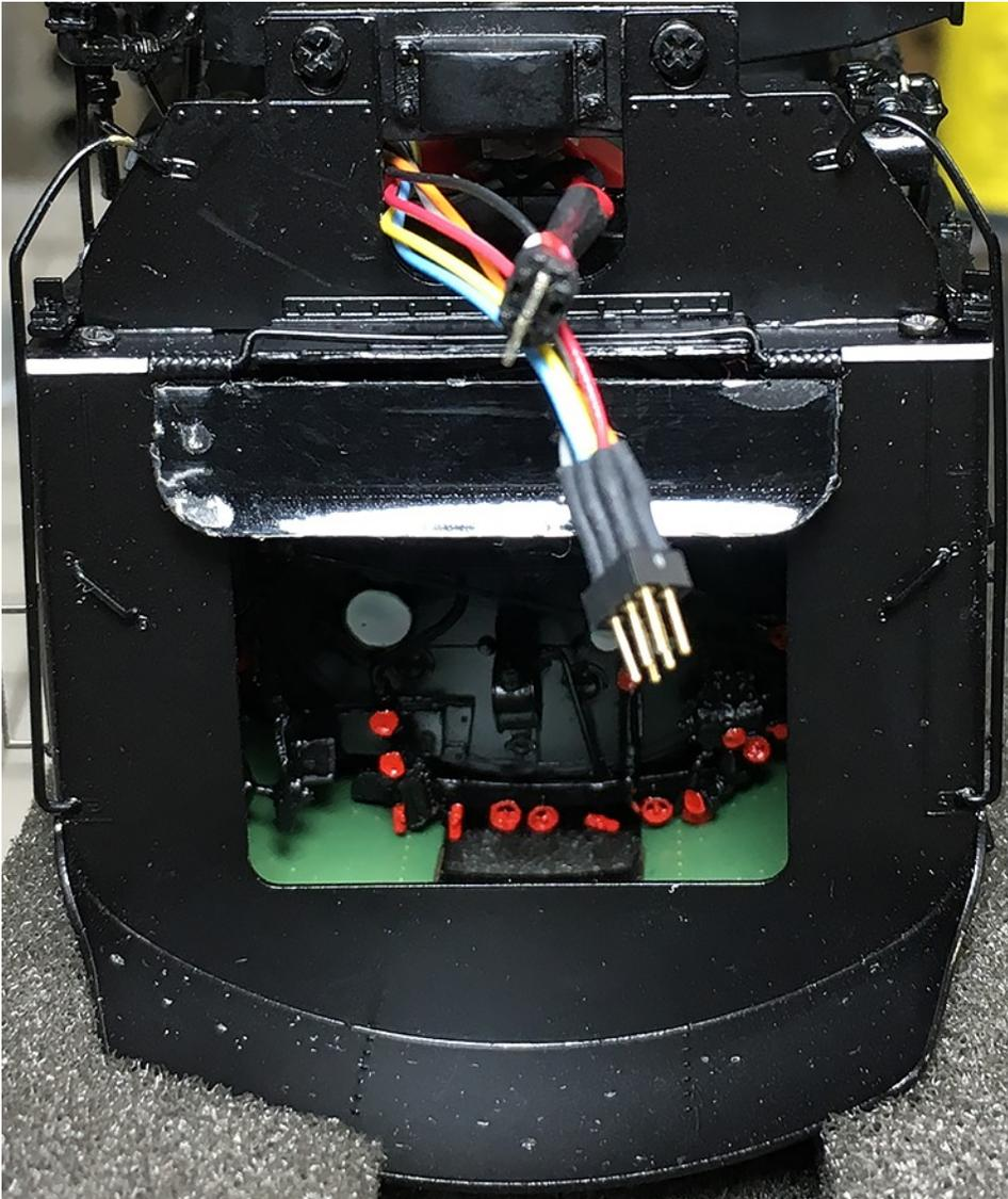
Here you can see the plugs coming out of the locomotive. The 2x3 mini connector will get heat shrunk before being delivered to make things neater and hide the colored wires. The smaller two pin connector carries the track power back to the decoder in the tender.
