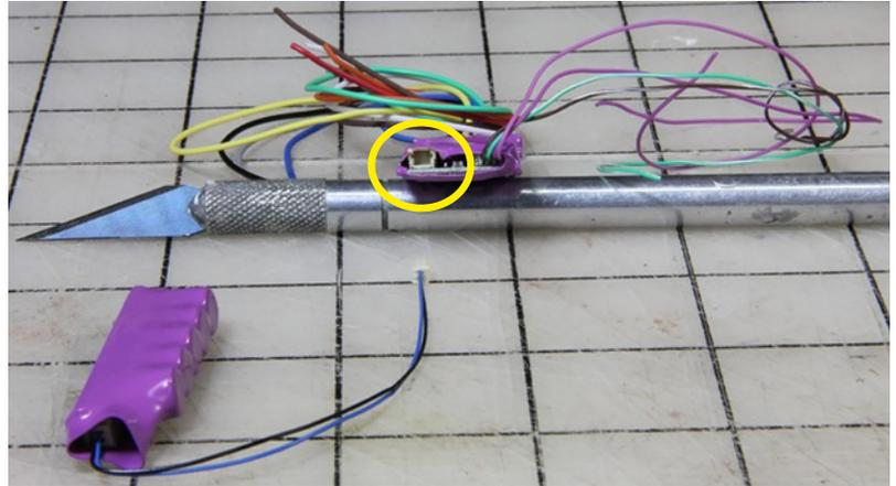
*Using an X-Acto, knife simply trim away the wrap which will allow the CurrentKeeper to be plugged in.*
