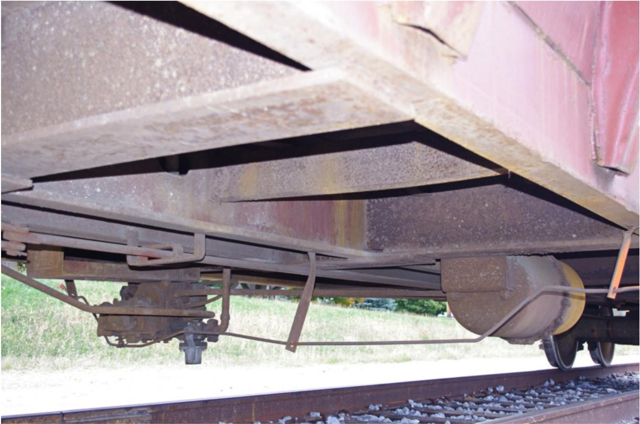
*ABOVE: Underbody and brake detail of a prototype Greenville gondola, MP 642902.
