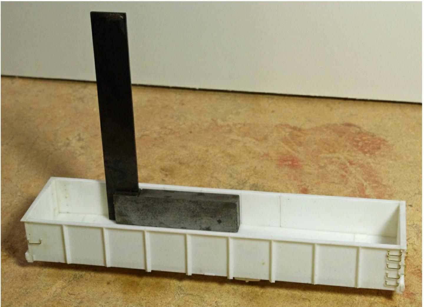
*To make sure the inside braces were located right and straight, I used my small square as shown. I used a fine mechanical pencil and marked lines on the inside of the car for reference.*
