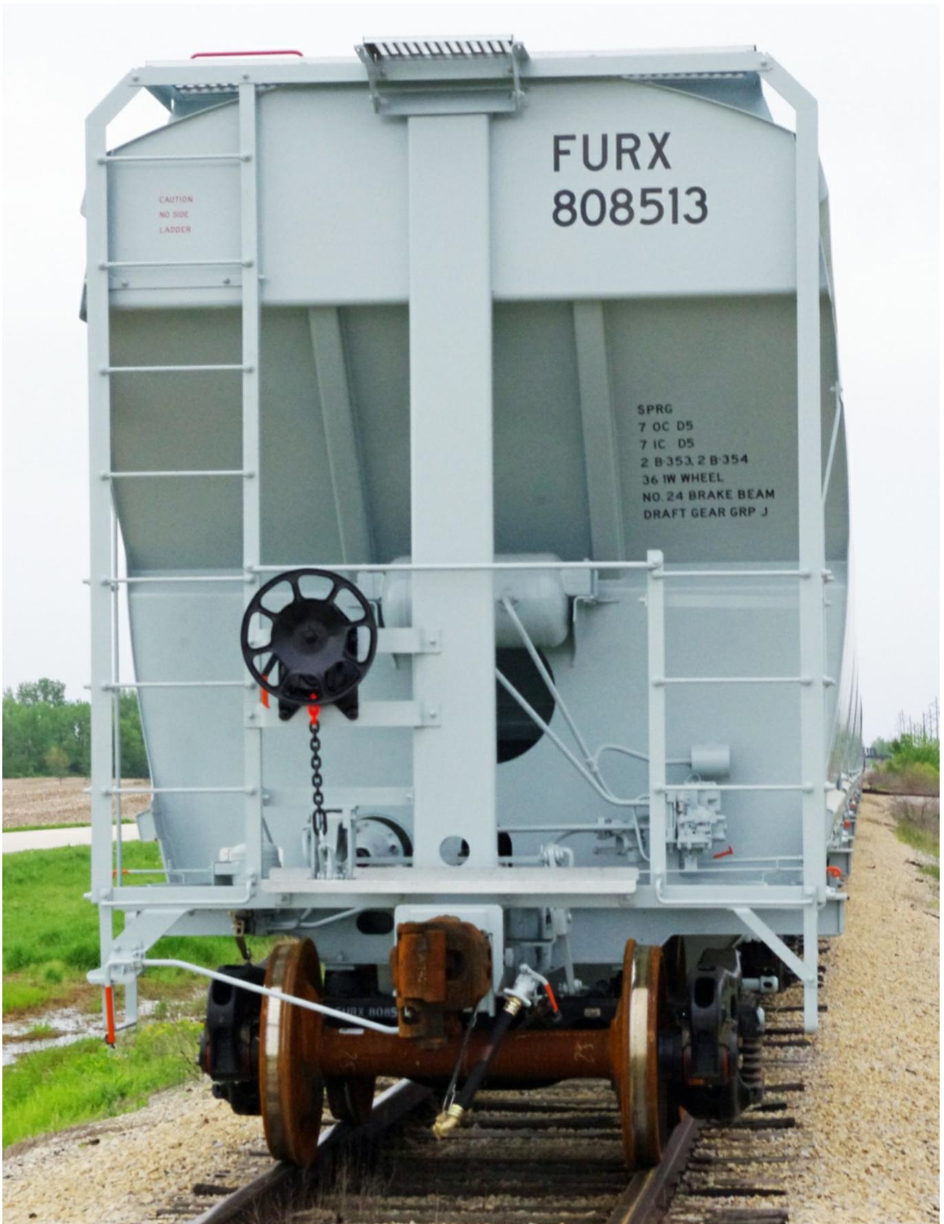
*Here is the B end of the car. Notice the black brake wheel and gear housing and the red tip on the cut lever and the air line valve. The brake rod to the other end of the car runs in a tunnel just above the center sill. The hole in the end support, just above the coupler, is to feed the brake rod through.*
