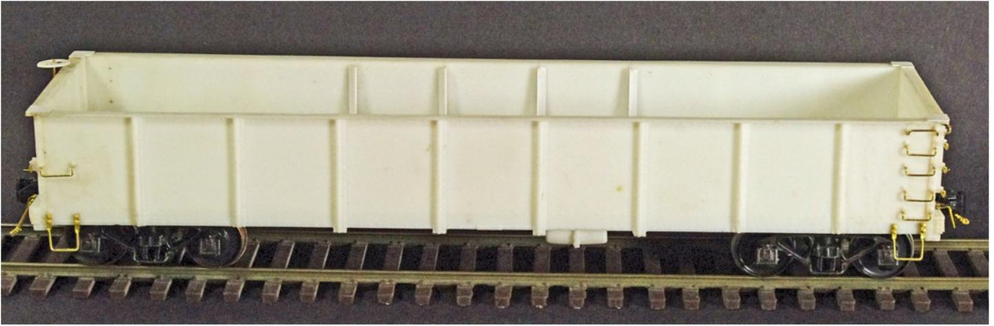
*Here is the finished car ready for paint. I made brass steps because they would be more durable than the cast steps that came with the model. Matt intends to operate a switching layout, and the cars will get a lot of handling.*
