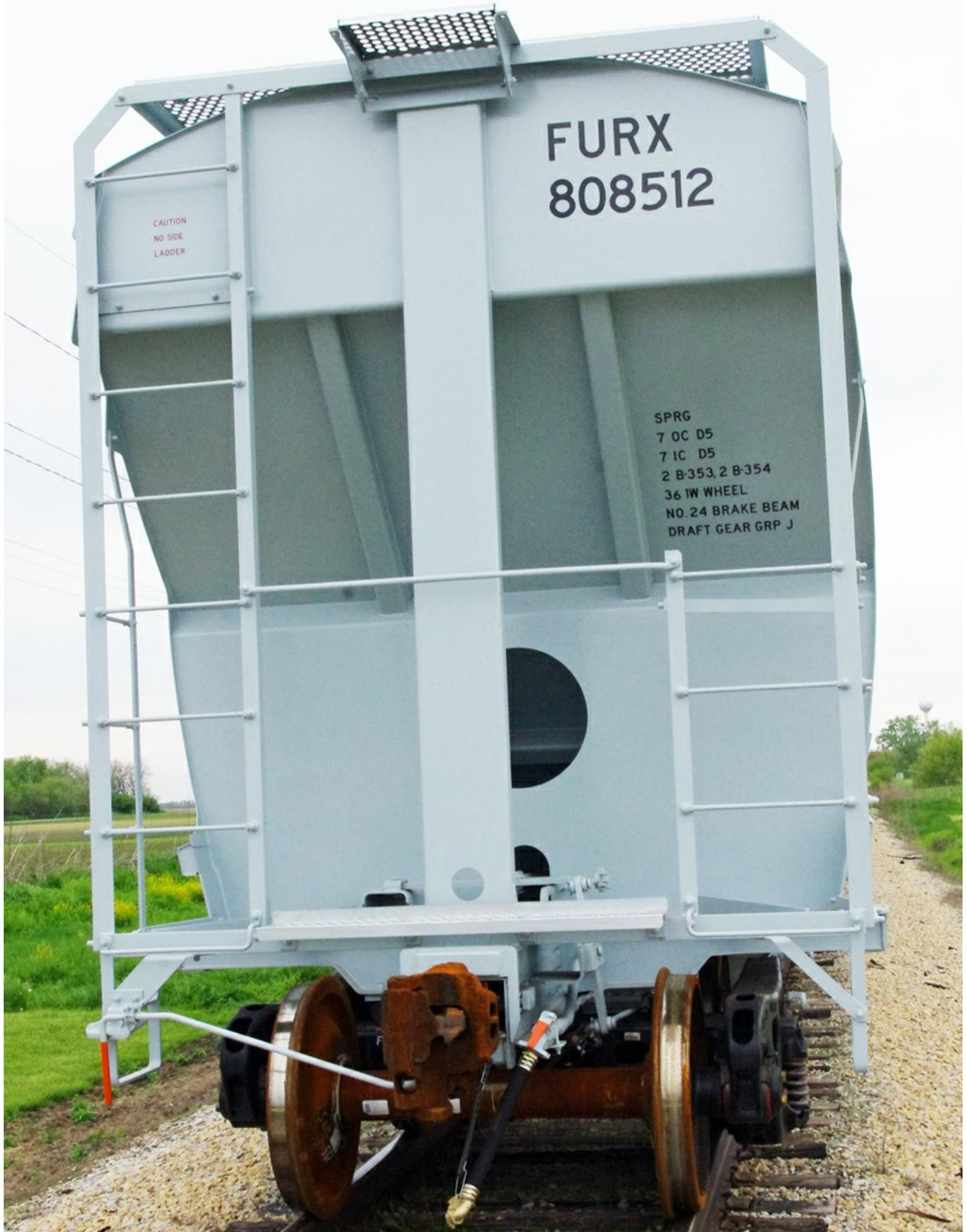
*This is the A end of the cars. Notice the lettering on the ends. The brake dead lever is located on this end of the car. The brake rod runs the length of the car in a tunnel just above the center sill. Notice the natural rust color of the wheels, axles, and couplers – not all parts are painted.*
