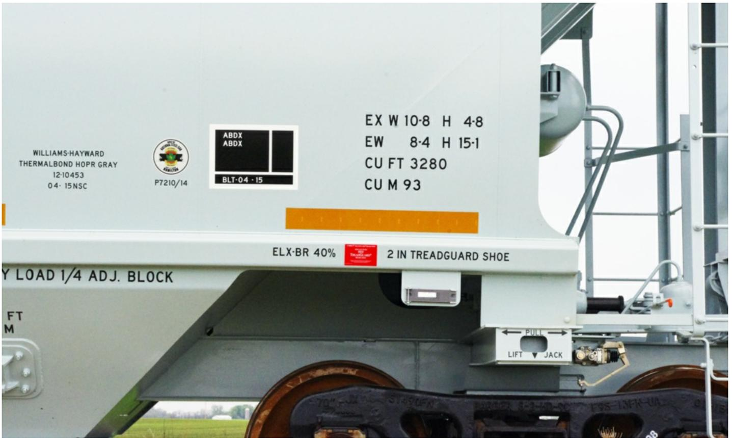
*Notice the car identification box under the “treadguard” lettering. These boxes house some electric circuits that transmit the car number to line side receivers for tracking the location of cars. This is a nice detail to add to a modern car.*
