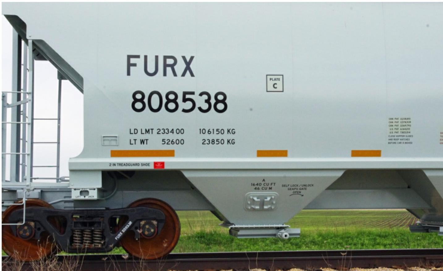
*The cars are all welded construction and could probably be scratch built out of styrene. Notice the color of the wheels. The couplers and wheels are not painted, but are a natural rust color. This is a nice touch that we can emulate on our models.*
