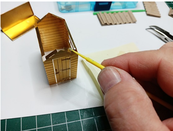
Once the walls were set, it was time to attach the sunroof section. A little CA and a microbrush worked great.
