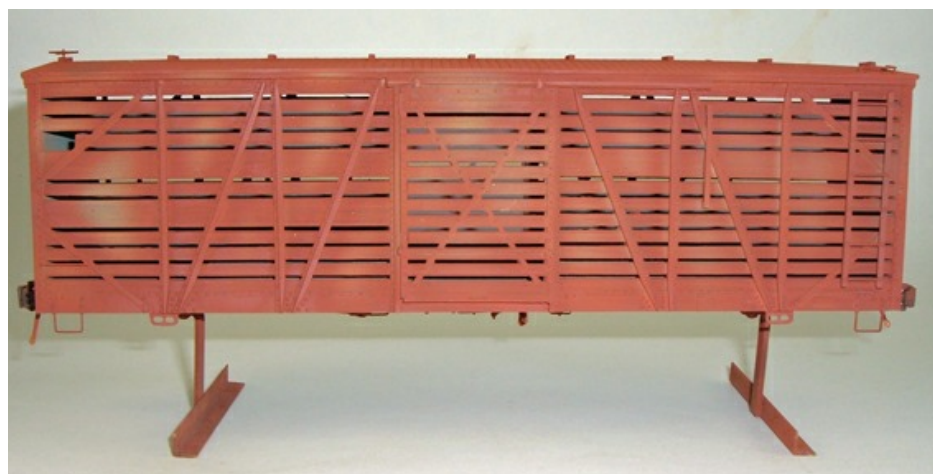
This is step three of the paint job. I have just sprayed the freight car red oxide color on. For this part, I concentrated on the metal parts of the car.
