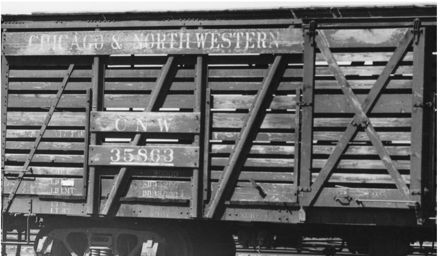
When I enlarged this photo, you could see the wood grain very clearly. The paint is worn off of this car. The lettering held up because the lettering paint is thicker and also protected the body paint.
