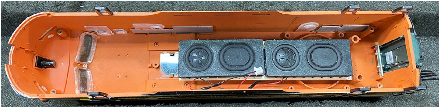
Tang Band speakers wired in series and attached to the styrene using carpet tape.
