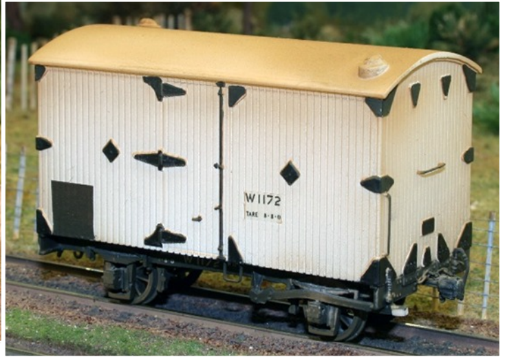
W10 wagon s scale 1/64 built on a commercial chassis the body is printed in one piece.
