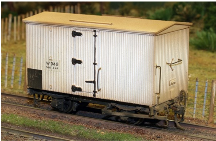
W5 wagon scale 1/64 built on a commercial chassis the body is printed in one piece.
