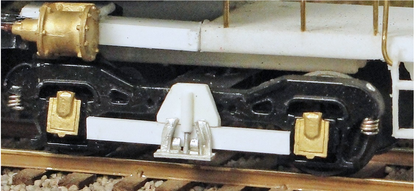
This view shows the completed third-rail shoe assembly on the pilot truck. The metal portion of the assembly is simply the bottom of a dummy switch stand! Dummy coil springs have been added to the ends of the PRR truck sideframes in order to match the appearance of the EP-3 truck.
