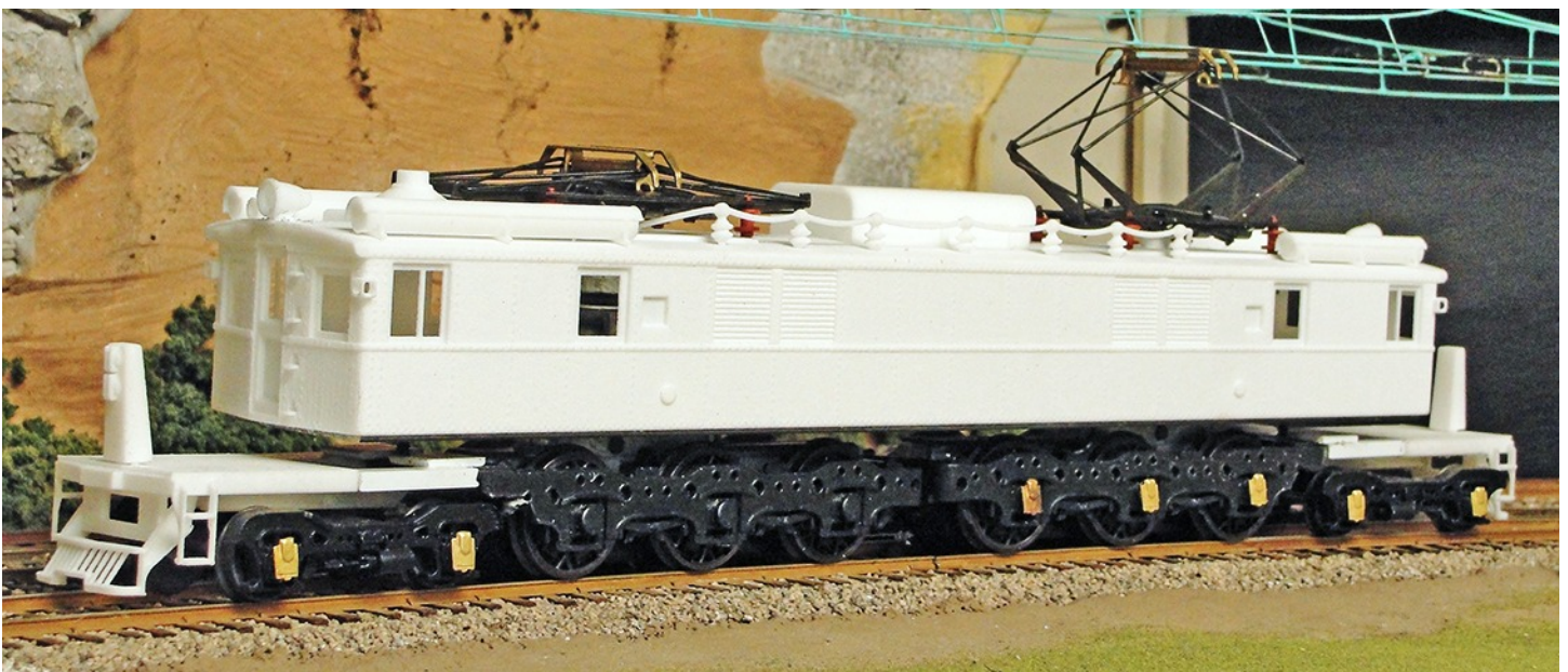
This early stage of test fitting verified that everything was properly placed. Plain brass journals, not yet completely installed, are copies of SSL&S parts.
