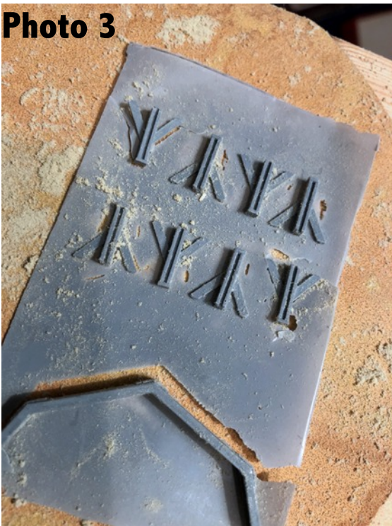
Photo 3 & 4: Partially through the sanding process and some of the parts are already coming free. Sanding resin this way can create a lot of dust, so it's best to work outside or over a waste bin of some kind. When complete, the parts will fall out and literally leave the “shadow” behind.
