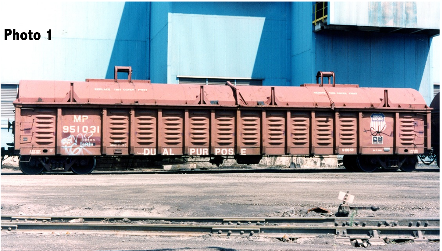
Photo 1: MP 951031, a 53 ft Greenville Gondola with load protecting covers in place. This car carries a UP herald, but retains its original Missouri Pacific reporting marks. Geneva, Utah, May 1994. Jim Rose photo, used with permission.
