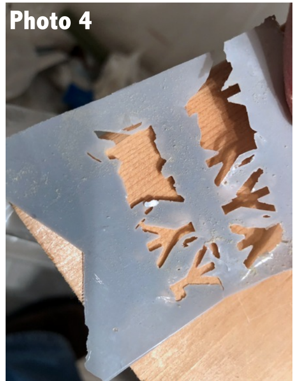
Photo 3 & 4: Partially through the sanding process and some of the parts are already coming free. Sanding resin this way can create a lot of dust, so it's best to work outside or over a waste bin of some kind. When complete, the parts will fall out and literally leave the “shadow” behind.
