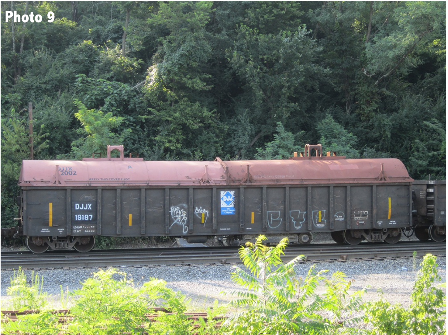
Photo 9: Prototype photo of Davis Joseph Transportation Inc., Thrall 2743 gondola DJJX 19187. Gondola is equipped with the coil cover being done by Pre-Size Model Specialties for Thrall 2742 gondolas. Ludlow, Kentucky, August 2019, photo courtesy Jim Kindraka.
