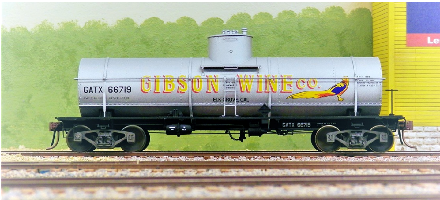
The Gibson Wine Co. tank car is built up of brass and styrene with decals from Protocraft.
