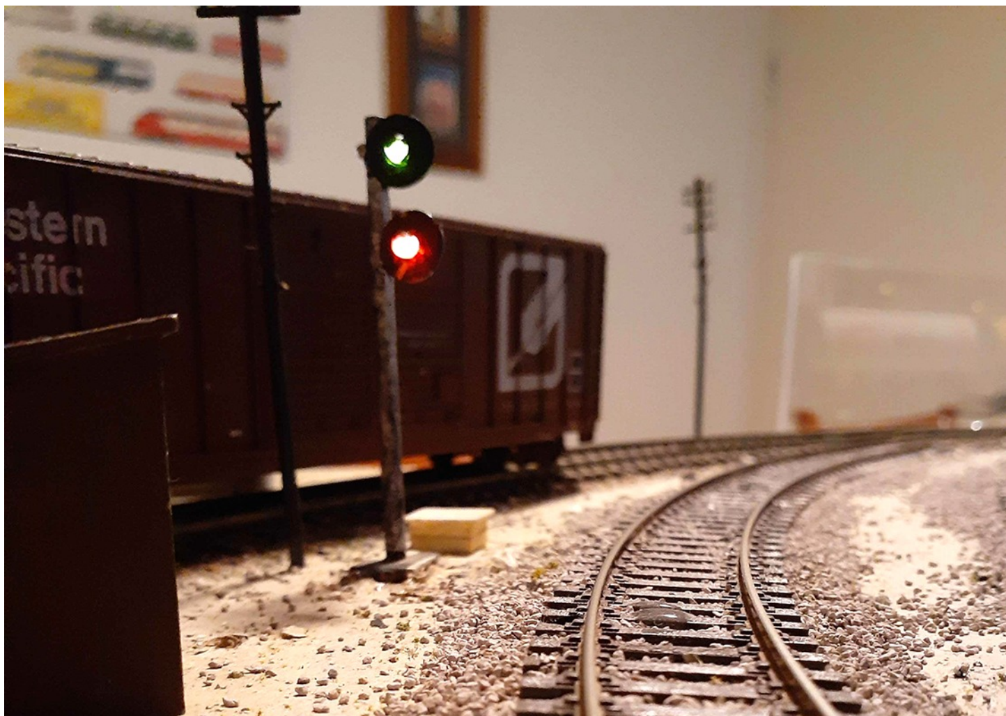
A double signal for the "intermediate stations". The bottom signal only uses the Red/Yellow aspect given it is only used for local movements.
