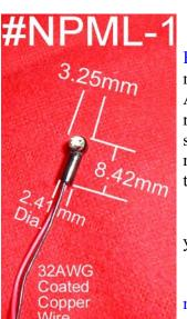
Dave from LBR Enterprises has a new marker light for 3/16 scale AF steamers. \$8.25 pr. with resistor attached plus free shipping in CONUS. There may be many uses for this in the scale world as well.
