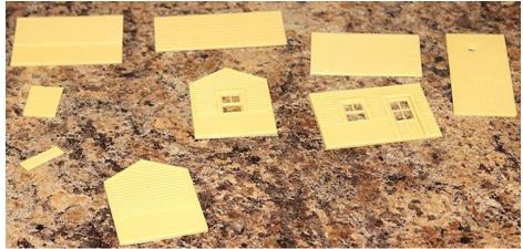
The parts were removed from the hot water and placed on the Formica countertop which is very flat. This was done because a few pieces were warped and needed to be straightened before sanding.
