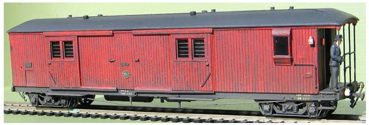
One of my scratchbuilt guards vans showing the steam loco soot and rain weathering.
