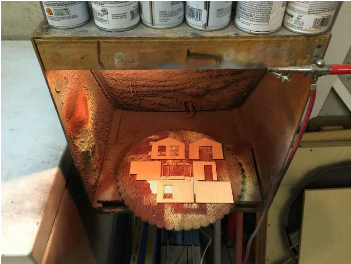
Above: I made a spray paint booth that vents outside with a blower. It has a light and a cake decorating turntable and a changeable furnace filter to knock paint drops out of the air.
