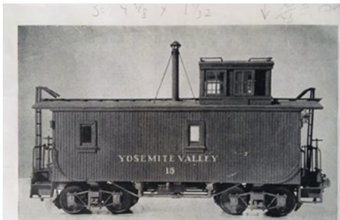
3-4 This unusually detailed S gauge caboose took Robert F. Shank of Los Angeles, Calif., an entire year to construct. It is equipped with seats, tables and a pot-bellied stove. The underside has all of the truss rodding of the prototype as well as the brake rigging. Bob worked from notes and photos taken from a full-size caboose. He spent a total of $2.68 for all the materials needed.
