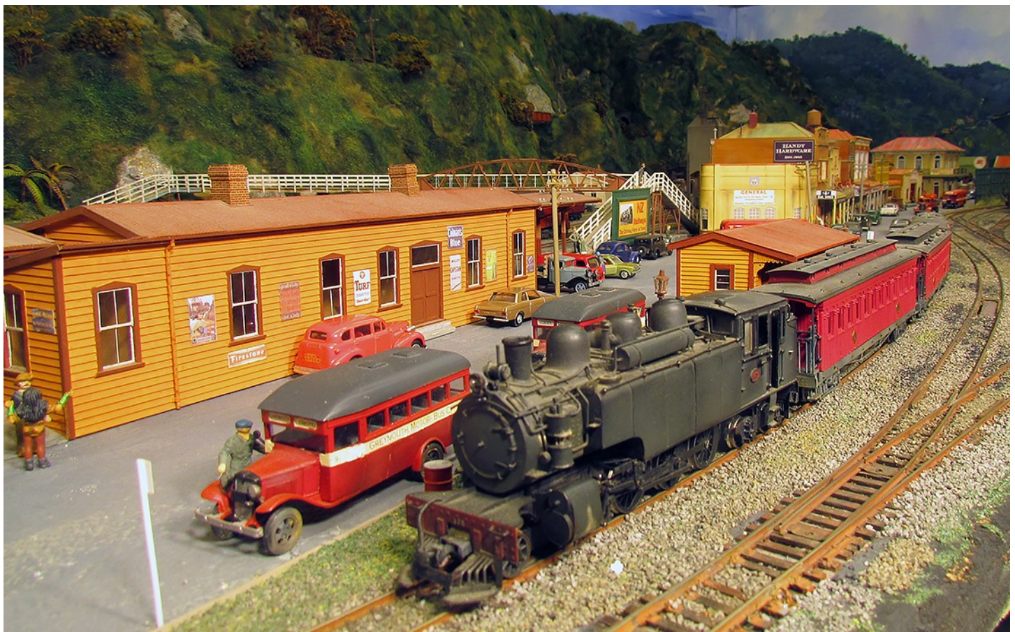
We376 a 4-6-4T, about to take a miners service up the incline to Rewanui from Greymouth's Riverside platform. The main station is at rear. Note the gap in the cowcatcher due to the "Fell" inclines centre rail for braking purposes. The Ford model B buses etc. are manufactured as kits by us. ( Railmaster Exports )
