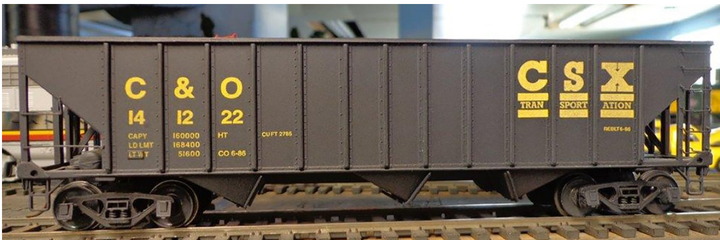
The basic model used as the starting point. The S Scale America H-39 triple hopper in a C&O - CSX paint scheme, sold by Des Plaines Hobbies. This particular model was chosen because several parts of the lettering could be kept on the final CSX coke hopper versions. Photo by Chuck West.
