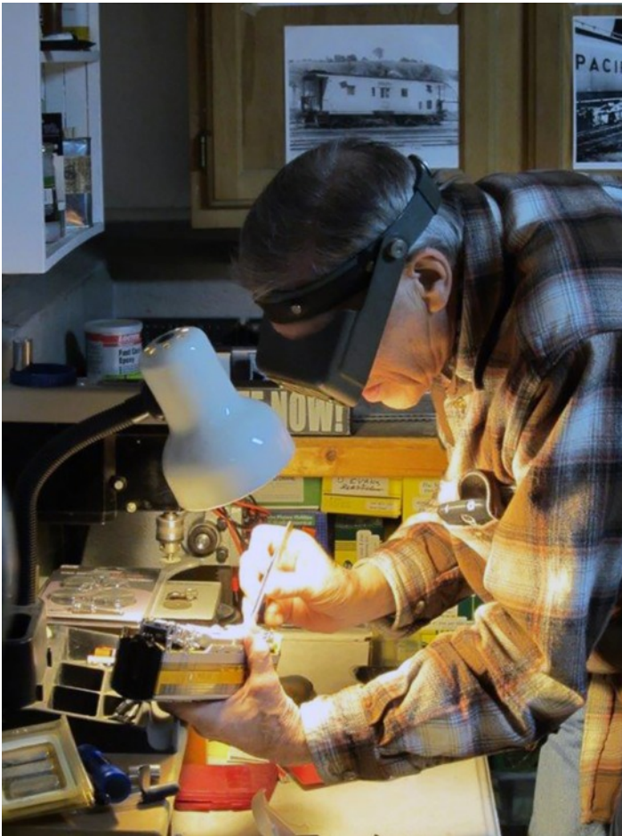
Chuck West dons his visor to adjust a wheel wiper on an SHS F7. Taking a close look with good lighting is an excellent way to find and repair little adjustments that separate operational issues from an otherwise smooth running model.
