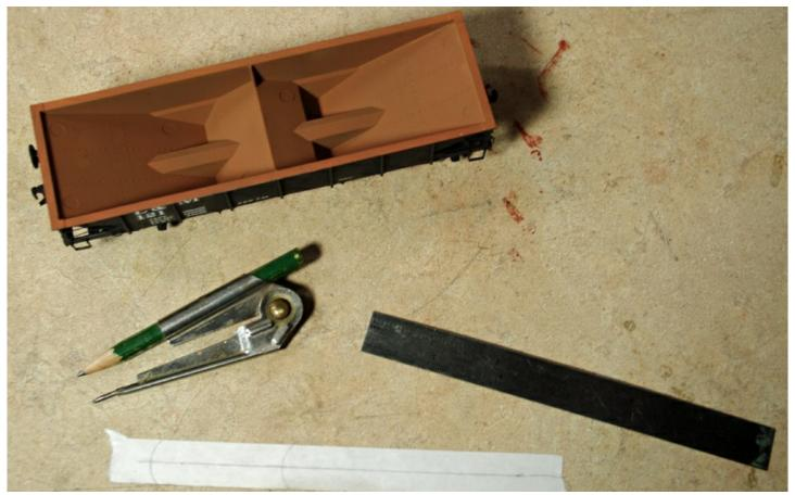
To lay out the curved lettering on the side of the car, I made some guides using painters tape. I drew a center line and then an arc. The centerline helped me find the center of the word, and that is where I started placing the decal lettering. I cut the tape with a knife.
