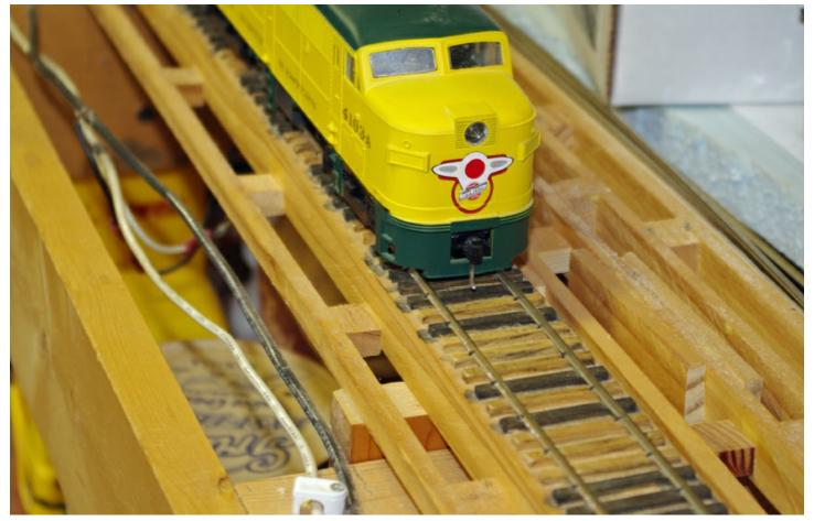
In this view you can see some of the spline construction. On the right is a track with no cap on the spline yet. See how Roy makes his roadbed with three splines and spacers. This saves time and wood. On the track with the locomotive, you can see the splines are only as wide as the ties, and there is a wood cap on the spline. Then there is a short spline. This short spline is to support the scenery.
