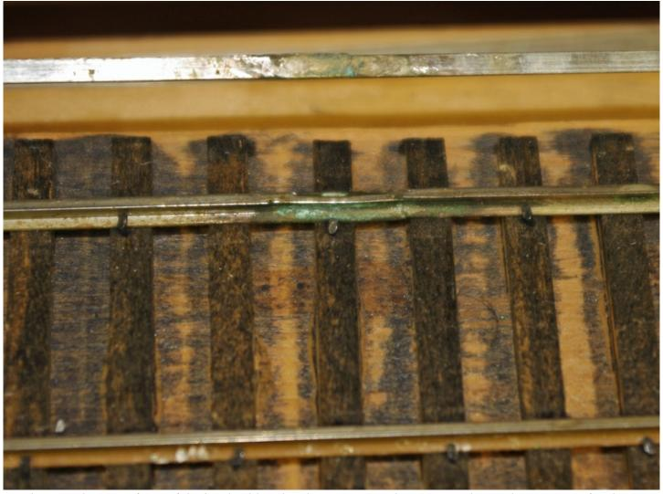
This is a close up of one of the hard soldered rail joints Roy makes. Next to the track is a piece of rail turned upside down so you can see the bottom of the joint.
