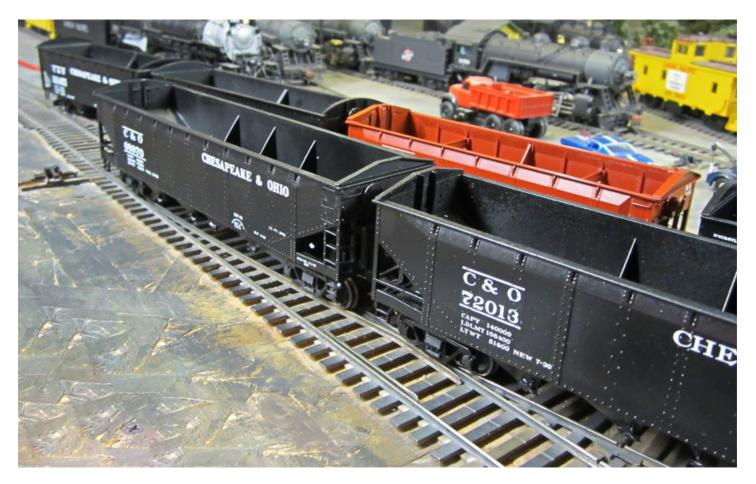
Here is a group of finished hoppers all with heap shields added sitting near the engine terminal on Chuck West's Des Plaines Valley layout. The group includes both 4-bay and 2-bay hoppers from a couple different S scale manufacturers, with both trapezoidal and radial heap shields added.
