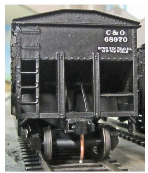
Photo 6: C&O 68970 is a completed 4-bay hopper with trapezoidal, or angular, heap shields applied. The prototype car was part of an order for 700 cars built by American Car & Foundry in 1928. With the heap shields, the car's capacity was 2968 cubic feet. The last of these class HT hoppers was retired in 1974.
