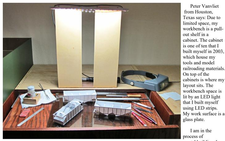
tools and model railroading materials. On top of the cabinets is where my layout sits. The workbench space is lit by an LED light that I built myself using LED strips. My work surface is a glass plate. I am in the process of scratchbuilding three PRR GLa two-bay hoppers in S-scale. These are built from styrene strip and sheet material. At the time of this photo, I was installing the
