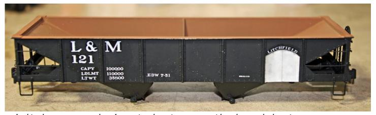
In this photo you can see how I am using the painters tape guide to lay out the lettering.
