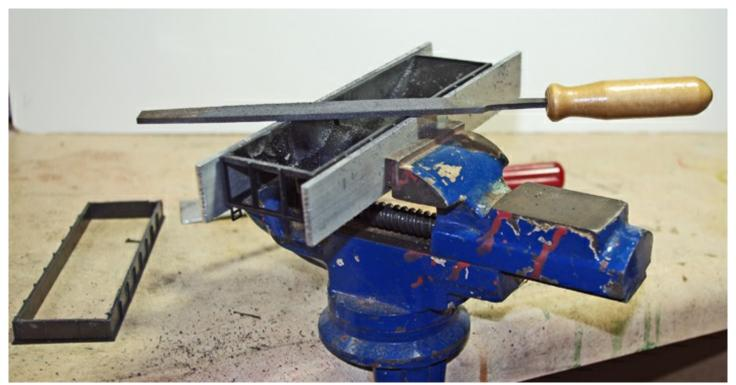
Cut the sides of the model first and then cut the ends. Then I used a file as shown to dress the top flat. The file worked good but did not give me the smooth surface I wanted
