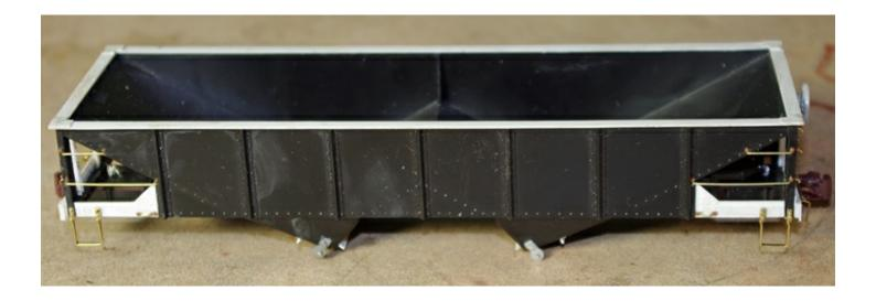
Here is the model ready for some paint. In the photo, there was a door mechanism on the sides of the hoppers. There was nothing on the model and I thought it needed something. I found some styrene brake wheel ratchets in the scrap box and just used them. I bent them, and ran a wire from side to side to act as the actuating rod. This is not the exact mechanism, but when painted it showed something there and that was good enough for my purposes.
