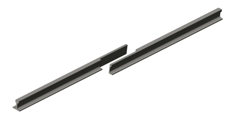
This is how Roy prepares the ends of his rail to make the lap joint. Each rail is notched halfway through for about 1/2" and then the rails are hard silver soldered together. This effectively makes one continuous piece of rail.
