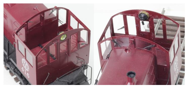
Sometimes we can cheat and not have to cut curves. You can see some of the straight angles I was able to use in the cab of this Alco S2. This unit is begging for an interior which is in the works.
