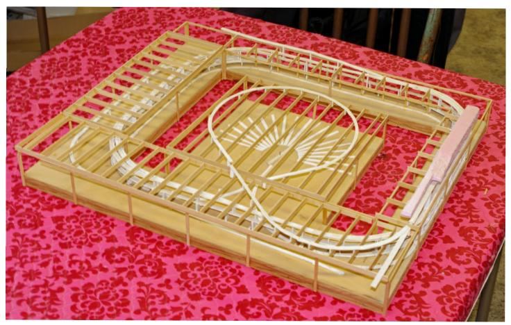
Roy Meissner built this model of his layout to help him visualize how the climbing tracks would get from the lower level to the upper level. By actually making a framing model, he was able to study how he would frame his layout.
