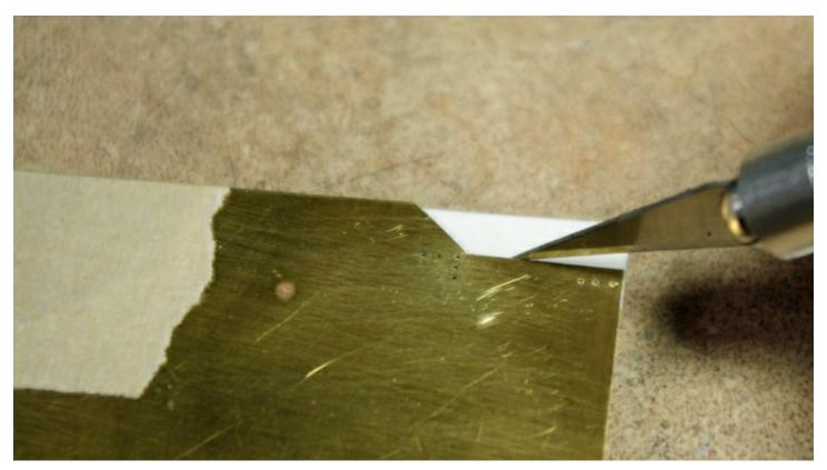
Here, I am trimming the styrene before removing it from the fixture. This worked out really well. The poked rivets held the part in alignment in the fixture, allowing me to cut a nice clean inside corner.
