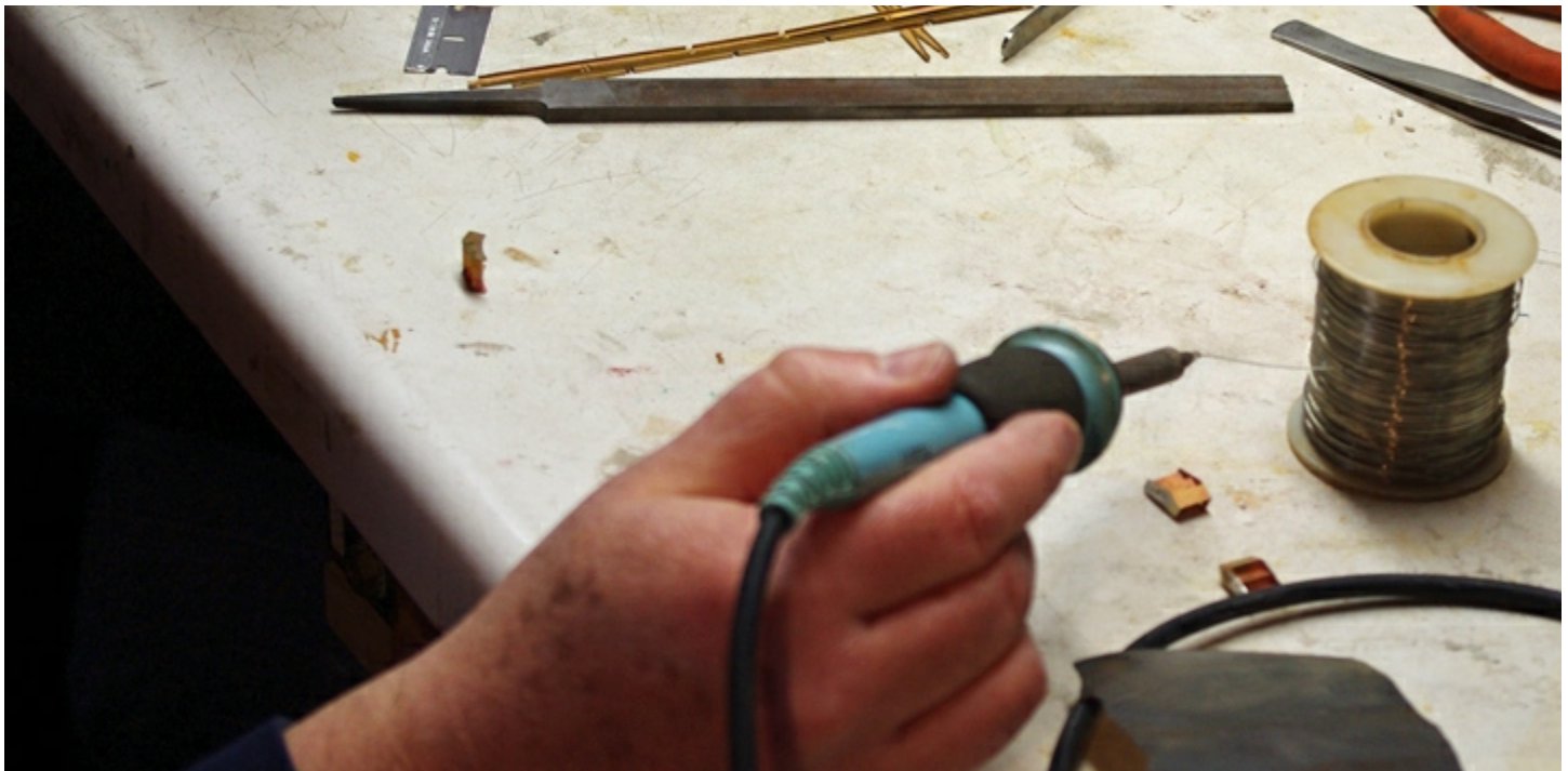
Here, Jim is going to solder the steps together for his S Scale Big Four caboose kit. One way to control how much solder gets on the part is to pick up a small amount on the tip of the iron like Jim is doing here. If you try to feed the solder into the work, you will end up with too much. This also frees up your other hand to hold something besides the solder. You can see some completed steps under the soldering iron. These are simple projects to learn on. The metal is thin and heats up easily.
