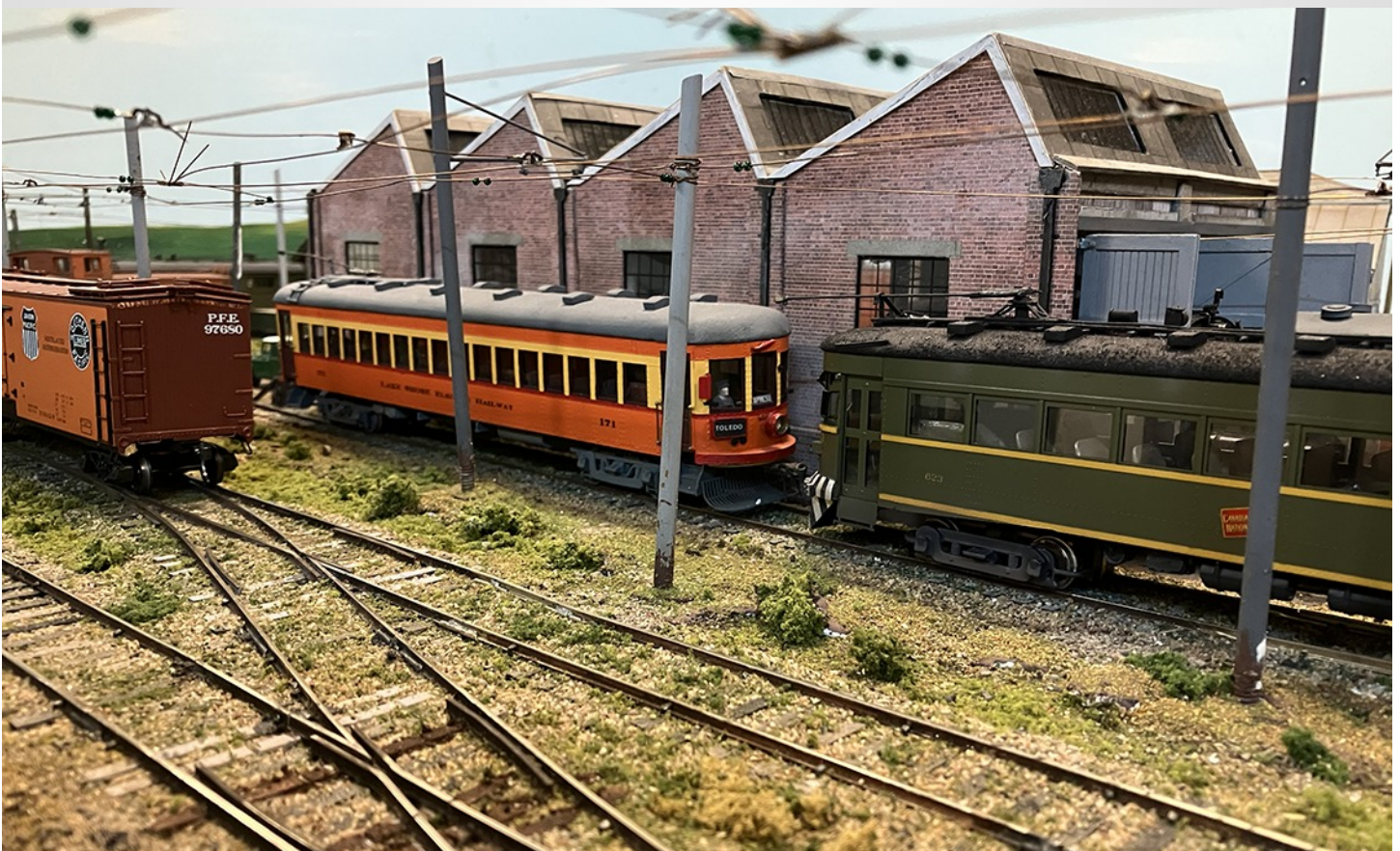
Below: Interurbans 623 and 171 at rest. Both cars are built from brass etchings and detailed with William's own castings. William designed the etching for 623, while 171 is a commercial etching. Both are DCC-powered and use Black Beetle power trucks.
