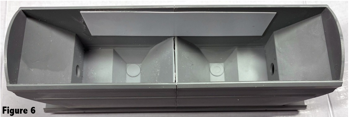
Figure 6: To add some strength to the car, I added some pieces of scrap .020 styrene which I made to fit the length of the car to get the most coverage possible.
