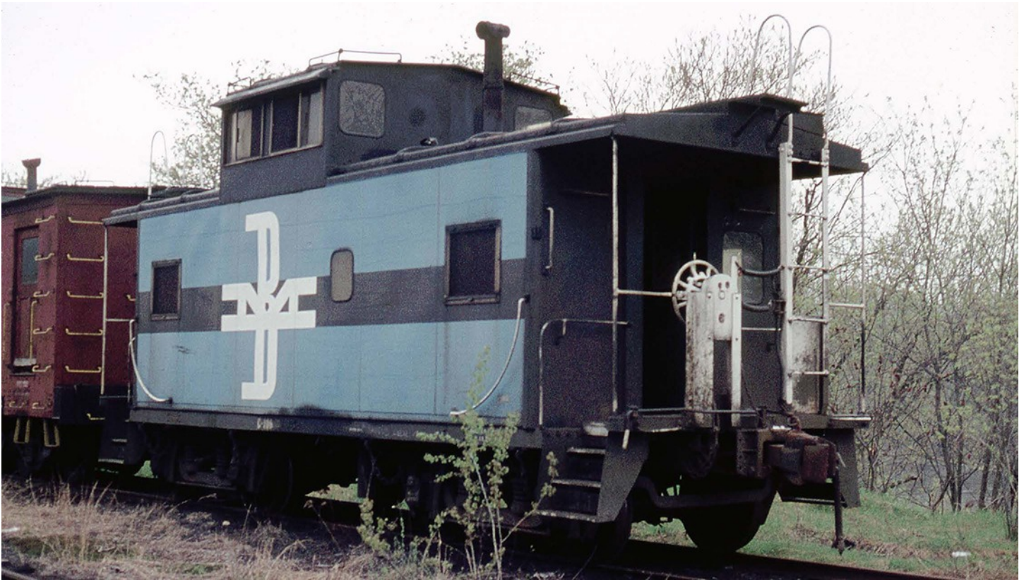
B&M buggy C-106 is at White River Jct., VT later on the same day, May 1, 1973, still in its original paint scheme. The only numbering on these cabooses in this scheme was on the sill, right next to the fill pipe for the oil stove. This often got covered with oil, making it very difficult to identify which caboose it was. Photo by Wayne D. Hills.
