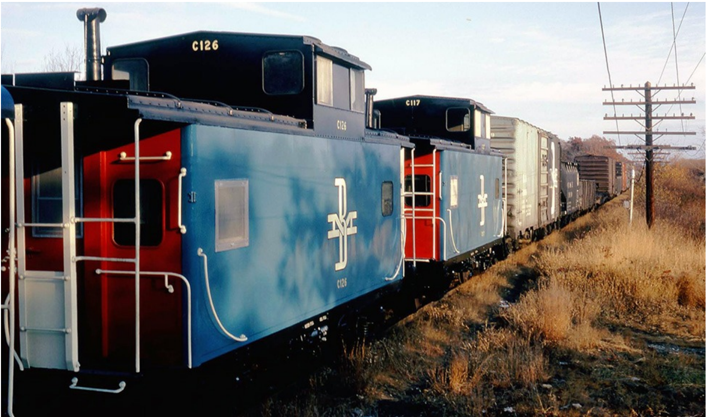
Cabooses C-117 and C-126 sit on the interchange track outside Billerica Shop in North Billerica, MA on November 10, 1972. These were the first two buggies to be painted in the new paint scheme with red ends and had new roller bearing trucks applied with axle driven generators. The axle driven generator experiment did not last long, and neither did C-126, being destroyed in a rear-end collision less than two weeks later. Photo by Wayne D. Hills.
