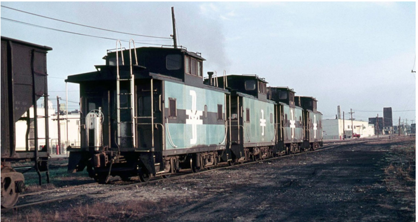
B&M buggies C-101, 105, 135 and 120 rest between assignments at Concord, NH on May 1, 1973. C-105 has been repainted with a blue body, but all four cars still retain their Commonwealth style 6 foot wheelbase trucks. Photo by Wayne D. Hills
