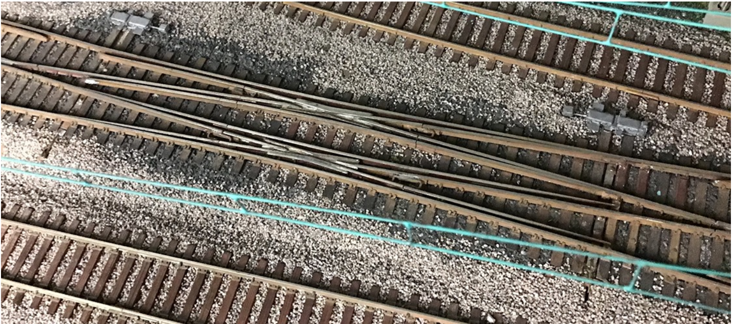
Dick built this No. 8 double-slip switch in 1962 as part of a passenger terminal yard throat. The 3 ft. by 8 ft. stand-alone throat module was under construction in Dick's rental living room. It originally had movable center frog points. However, when Dick installed the unit in his present layout, mechanizing the frog points was too complex, so he replaced the frogs with rigid ones. This is the only visible use of code 125 rail on the layout, All other track is codes 100, 83, and 70.
