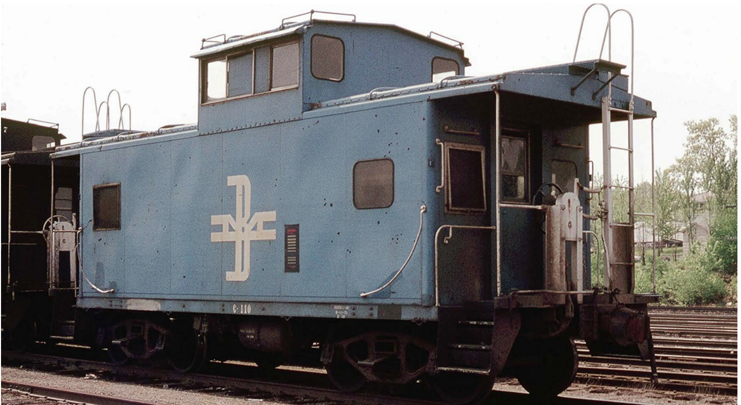
B&M C-110 sits in the yard at Nashua, NH on May 13, 1973. This caboose received a shopping sometime prior to its lube date of 2-18-71, at which time it received Barber-Bettendorf style caboose trucks with leaf springs and a blue paint job with a smaller herald. Photo by Wayne D. Hills.
