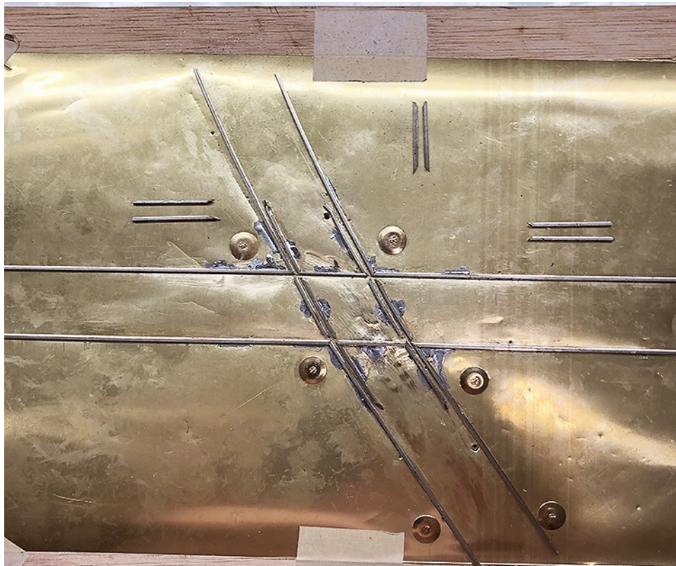
Below: In the next step, I install the guard rails for the stock rails and the diamond rails.
