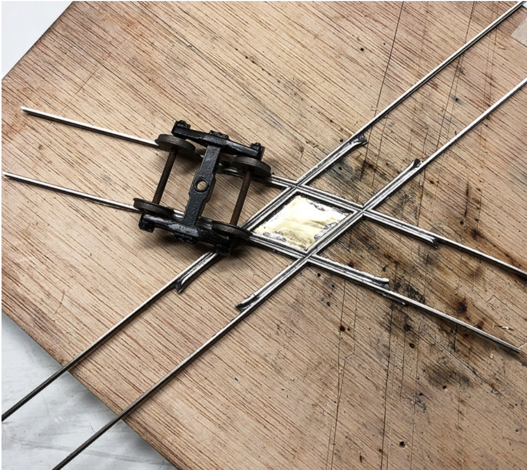
Above: I leave the foil in the diamond until I have cleaned and inspected the crossing. Below: Once everything checks out, I flip the crossing over and remove the foil from the bottom of the rails.
