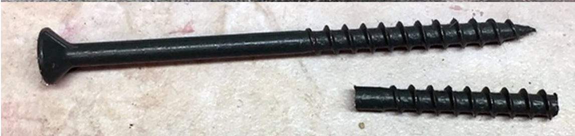
Deck screws were cut with a hack saw to create auger sections.
