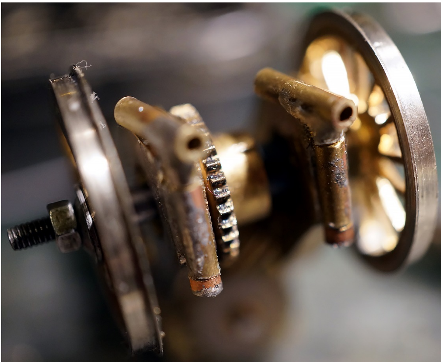
The king pin assemblies added to the motor gear box unit
