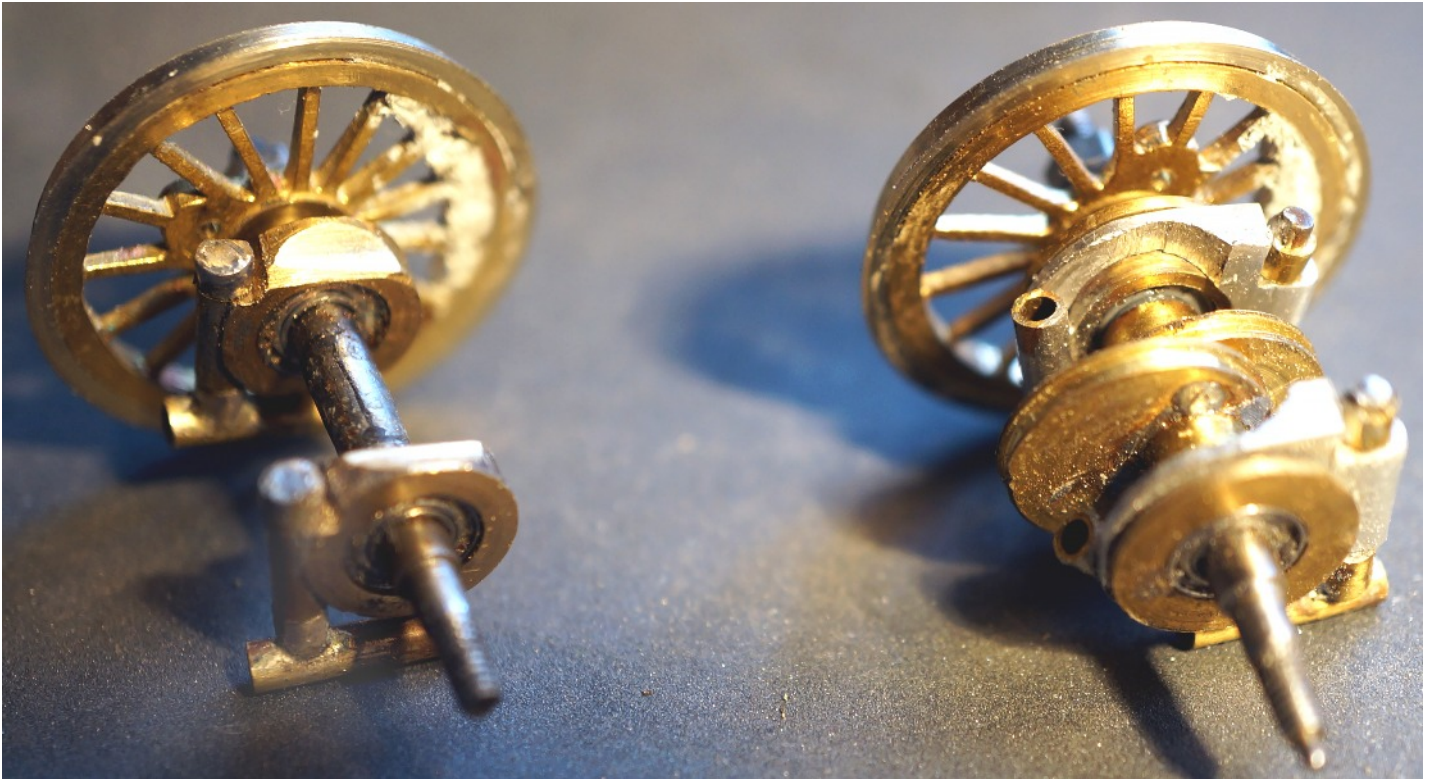
The front and middle axle and axlebox assemblies.
