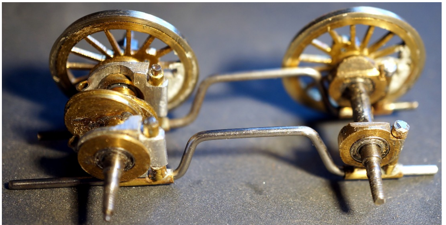
Trial assembly of the front and middle axles and the compensation beams.
