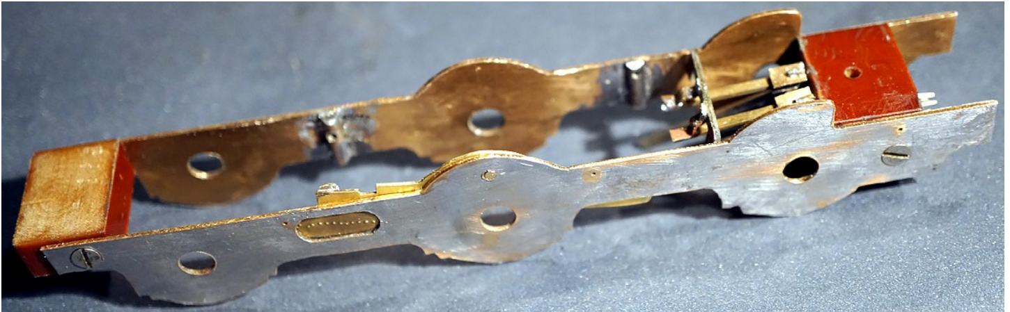
These photos show the attachments for the levers and the fifth lever pivoted at its mid-point with attachments for the other levers at its ends. This shows where I goofed, the pivots should have been in line with the axles.
