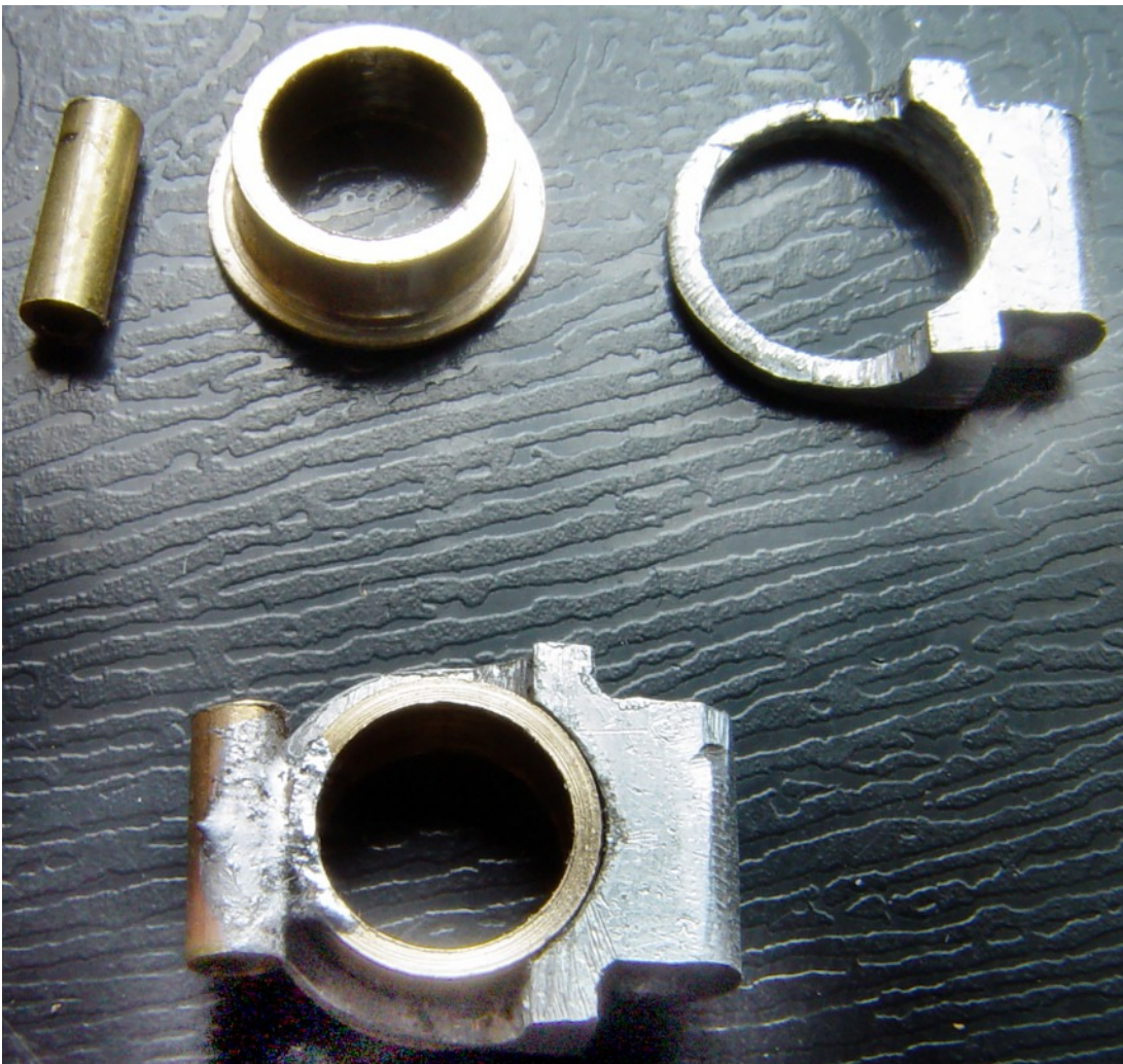
The hinged axlebox for the middle axle. The right hand component is made of Dural to ensure the whole thing doesn't solder up solid while getting a good solder joint between the tube and the brass bush.
