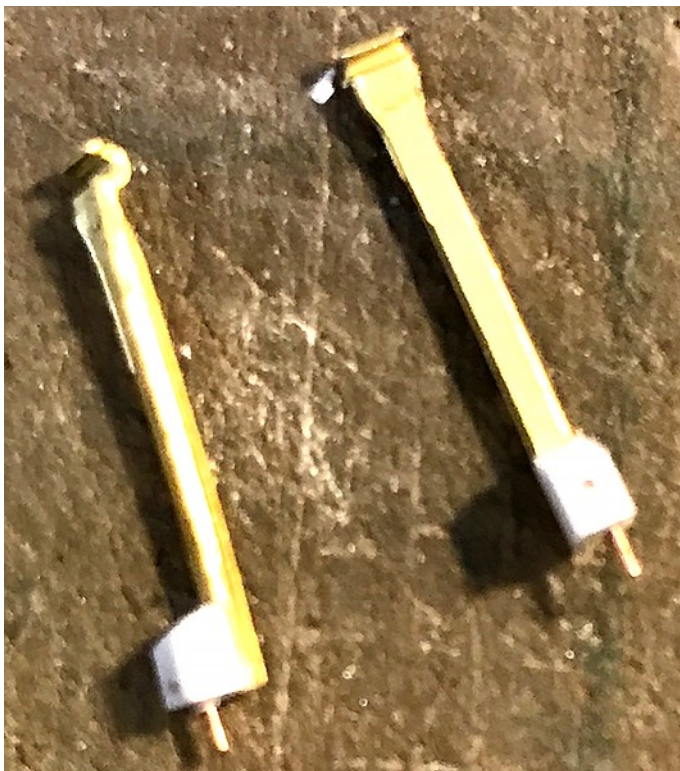
Photo 38 - The modified inboard stanchions are cut to length, and a small trapezoidal piece of 0.060" square styrene is secured to the back of the stanchion with a brass wire pin inserted into a hole drilled into the back of the stanchion and the styrene block. A second pin extends from the bottom of the styrene block to secure it to the deck. Do not attempt to merely glue the stanchion to the deck. It will not be secure and could be easily broken.
