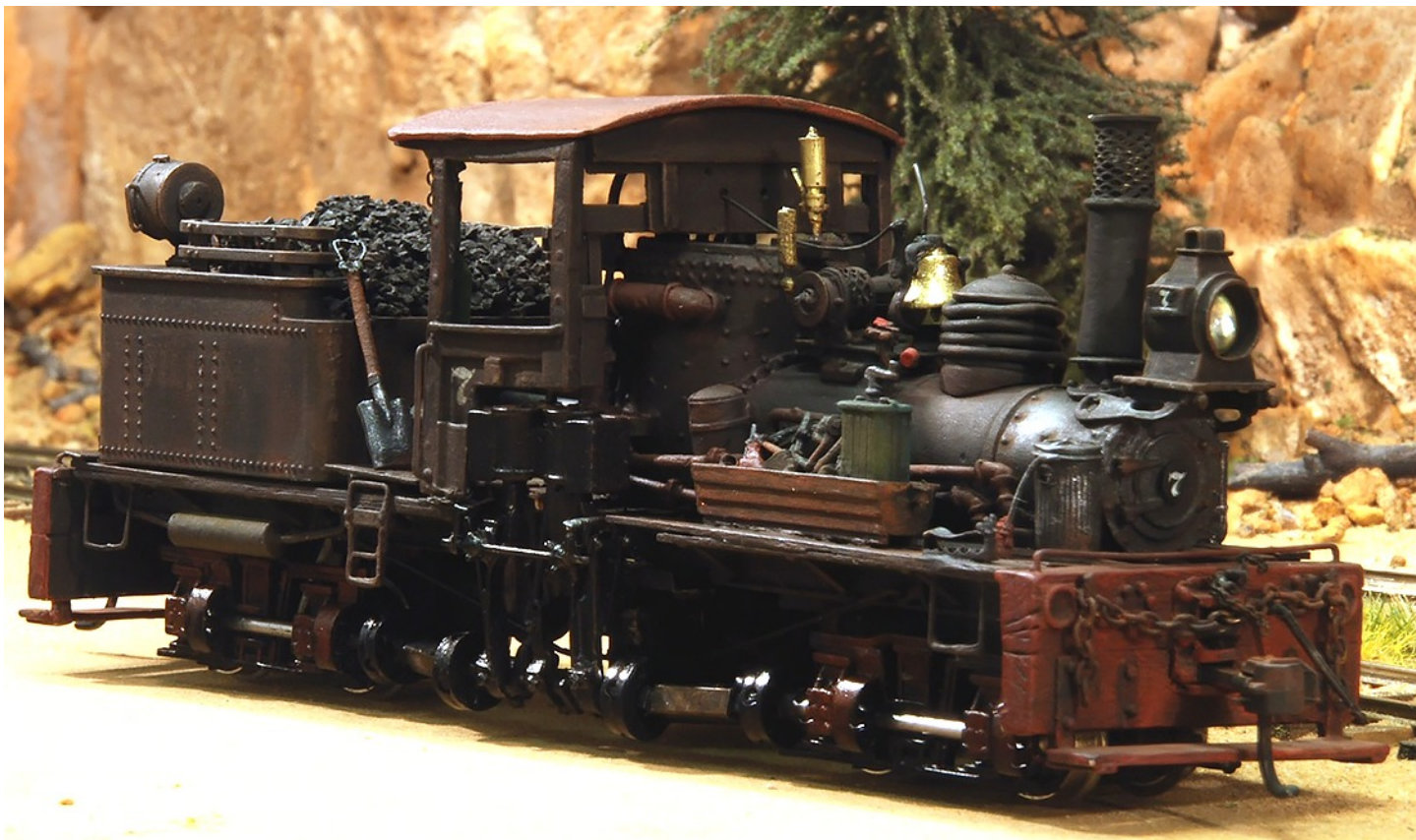
A HO On3 MDC shay with NWSL re-gearing and can motor converted to Sn3 detailed interior.
