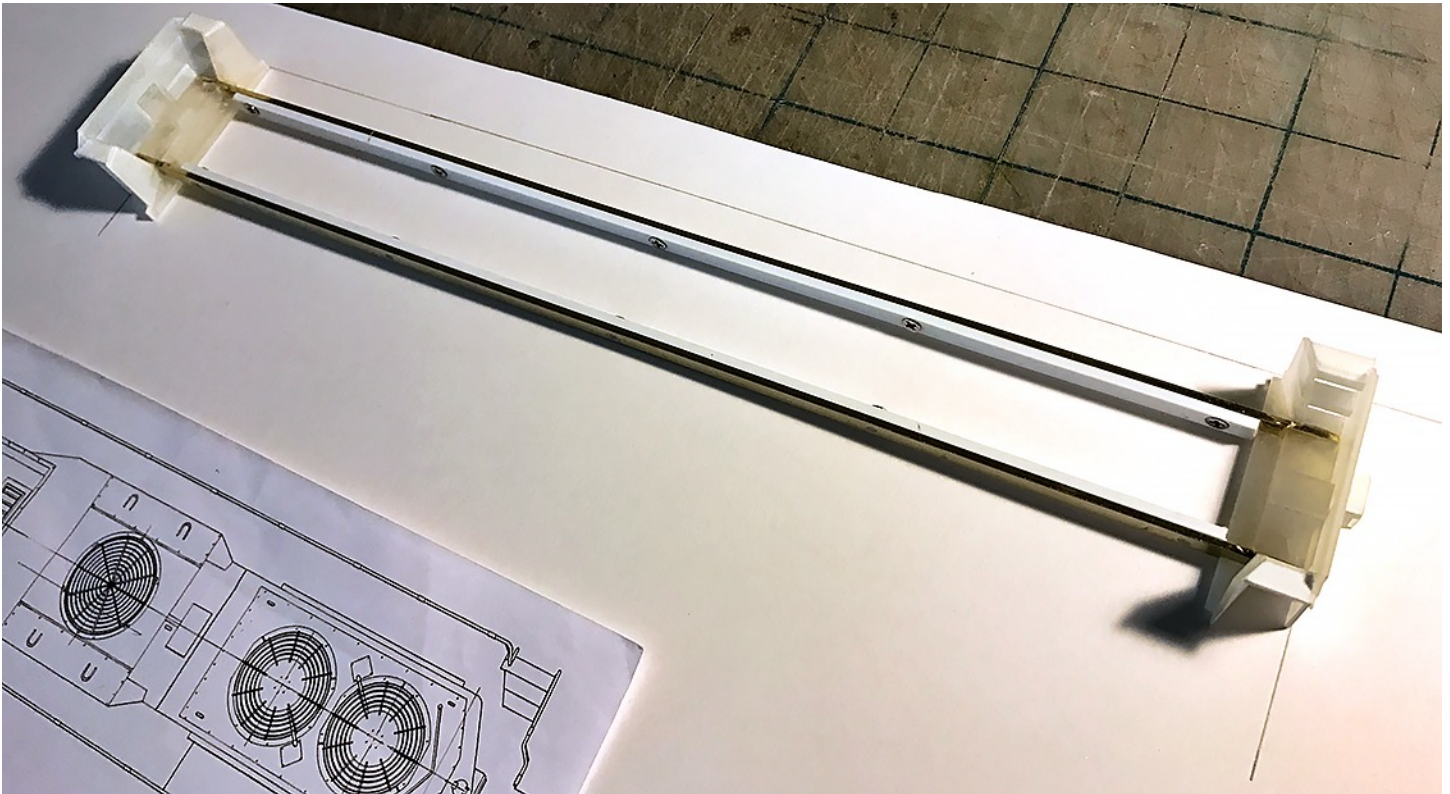
Photo 7 - Cut the deck from a sheet of 0.600" thick styrene the same width as the back of the step well and long enough to span from the end of the step well deck on one pilot to the other. There is a lip cast onto the pilot/step well print to support the edge of the styrene deck that keeps it flush the deck on top of the pilot. Use styrene cement to attach the deck to the styrene strip part of the composite floor beam and CA-type to attach the deck to the lip on the pilot/step well piece. (Note: this frame uses the modified 1/4" deep bars.)
