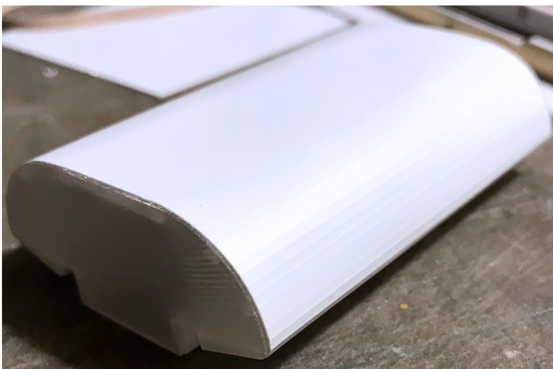
Photo 16- This photo shows the completed tank. Note how the edge of the wrapper meets flush with the tank end. There will be visible lines created by the V-grooves on the surface of the wrapper. This actually occurs on the prototype as well. This is a good time to test first the fuel tank by positioning it between the frame members at the correct location. Do not glue the tank to the frame at this time.
