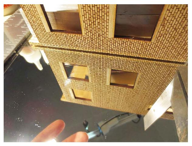
Photos showing how the mirror surface helps maintain a square assembly and allows one to see the joint for flat assembly.
