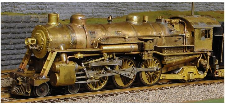
Fig. 7. Here we see much of the detail added after I resumed this project. Particularly evident are the water piping, air tank and its support cleats, boiler steps, sand piping, booster piping, and running boards (footplates for you Brits). The firebox now has a bottom (ash pan). Air piping is yet to be installed. The handrails will go on last, after the engineer's side is finished.
