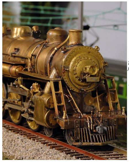
Fig. 8. This view shows the nearly completed front end. Note the air piping, pilot support struts, classification lamps, and booster exhaust pipe behind the stack. The loco is really filthy at this point, mainly from brass filings clinging to soldering flux residue. After completion, the loco will be disassembled and everything except the drive train and the plastic tender shell will be cleaned and carefully scrubbed in a lacquer thinner bath.
