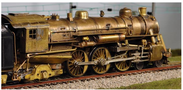
Fig. 9. Here's an engineer's side view after the power reverse, air distribution valve (above the power reverse), and air piping have been installed. The cab roof hatch is also visible in this shot.
