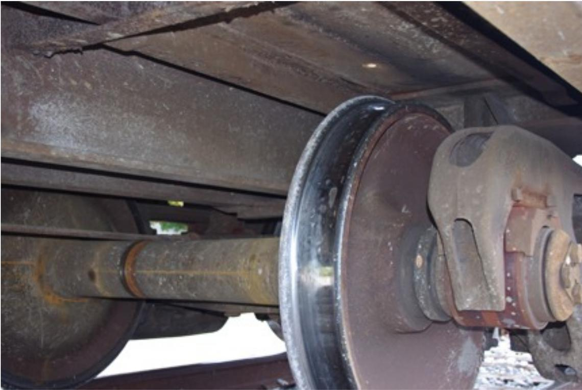
*Underbody and brake detail of a prototype Greenville gondola, MP 642902. The photo shows where the brake rod is rubbing on the axle. Photo by Glenn Guerra.*
