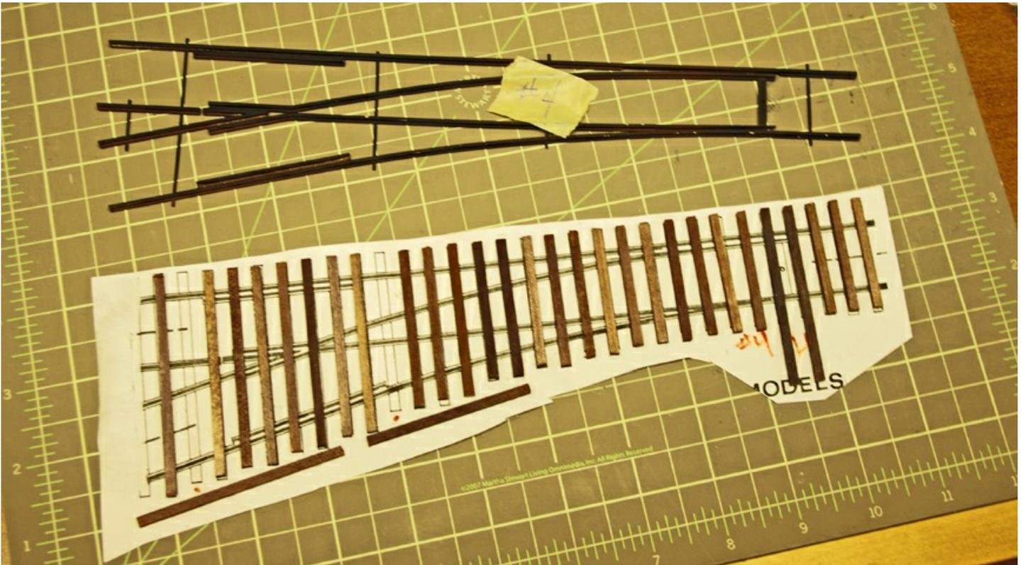
*Gaylord starts with Old Pullman switch kits. The rails are soldered together when they come from the factory. Gaylord glues the ties to the paper template first and then glues the rails to the ties. Now, he has a complete switch that can be moved around on the layout for alignment. I thought this was a good idea.*
