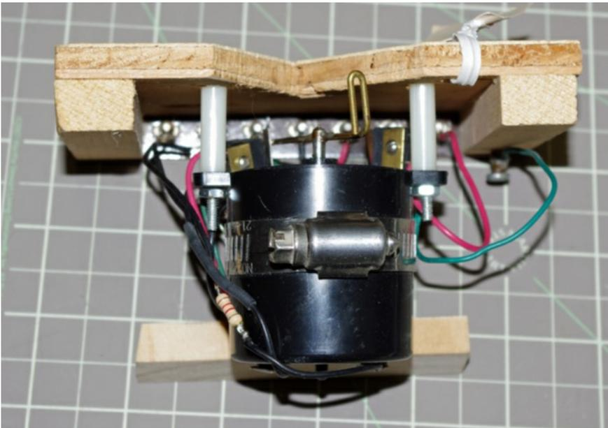
*Gaylord uses gear motors for switch machines on the main line. He mounts the motor and electrical connections on a block like this. The clamp around the motor holds limit switches that determine the throw of the switch. The biggest advantage to all of this is that it can be adjusted and assembled on the work bench, not while you are crawling around under the layout*
