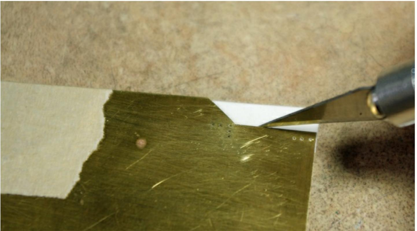
*Here, I am trimming the styrene before removing it from the fixture. This worked out really well. The poked rivets held the part in alignment in the fixture, allowing me to cut a nice clean inside corner.*
