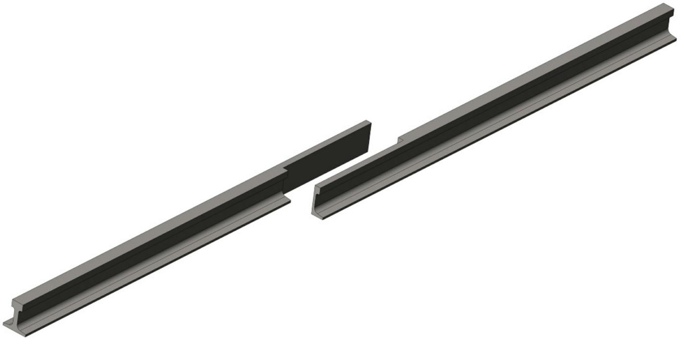
*This is how Roy prepares the ends of his rail to make the lap joint. Each rail is notched halfway through for about 1/2" and then the rails are hard silver soldered together. This effectively makes one continuous piece of rail.*
