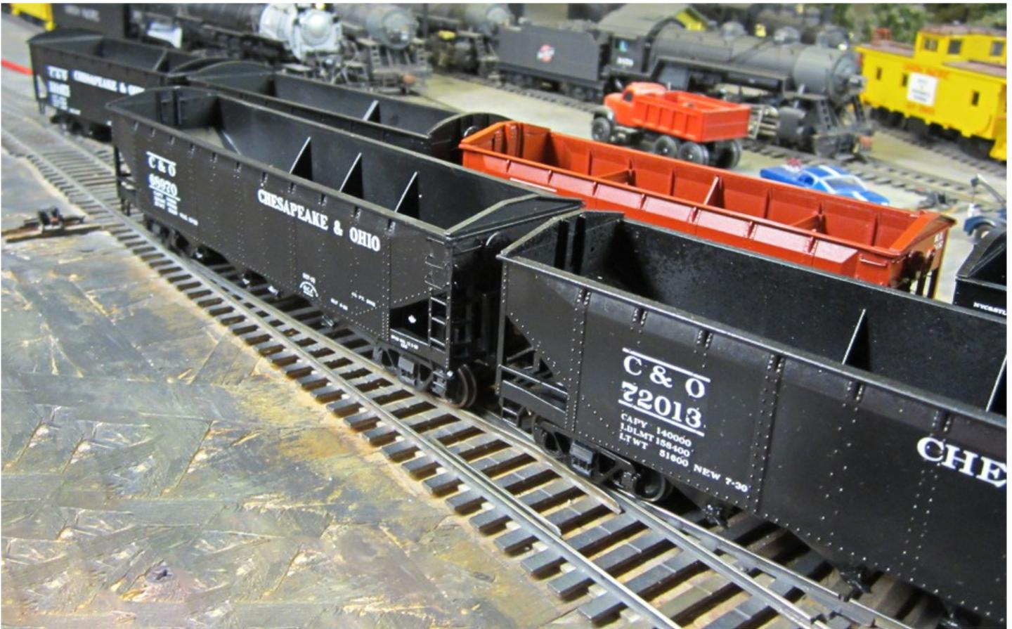
*Here is a group of finished hoppers all with heap shields added sitting near the engine terminal on Chuck West's Des Plaines Valley layout. The group includes both 4-bay and 2-bay hoppers from a couple different S scale manufacturers, with both trapezoidal and radial heap shields added.*
