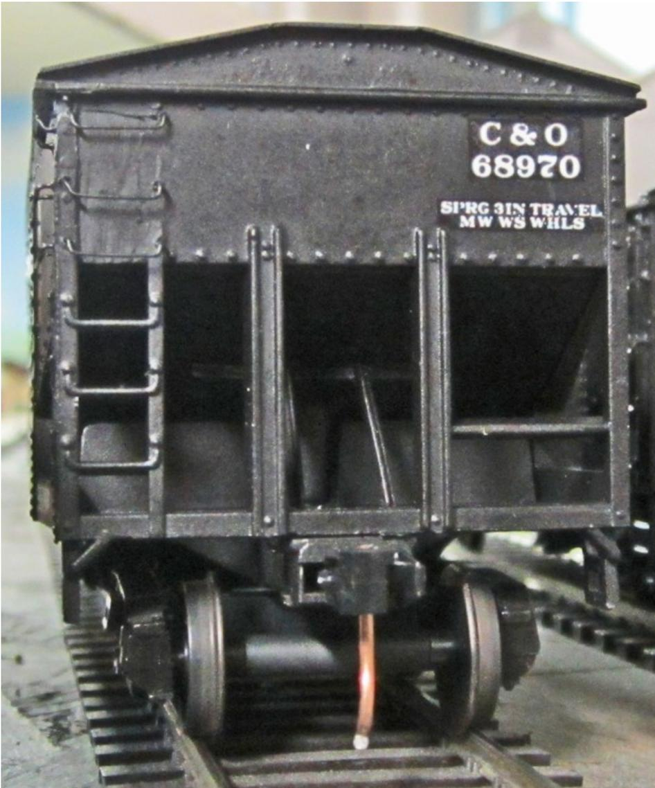
Photo 6: C&O 68970 is a completed 4-bay hopper with trapezoidal, or angular, heap shields applied. The prototype car was part of an order for 700 cars built by American Car & Foundry in 1928. With the heap shields, the car's capacity was 2968 cubic feet. The last of these class HT hoppers was retired in 1974.
