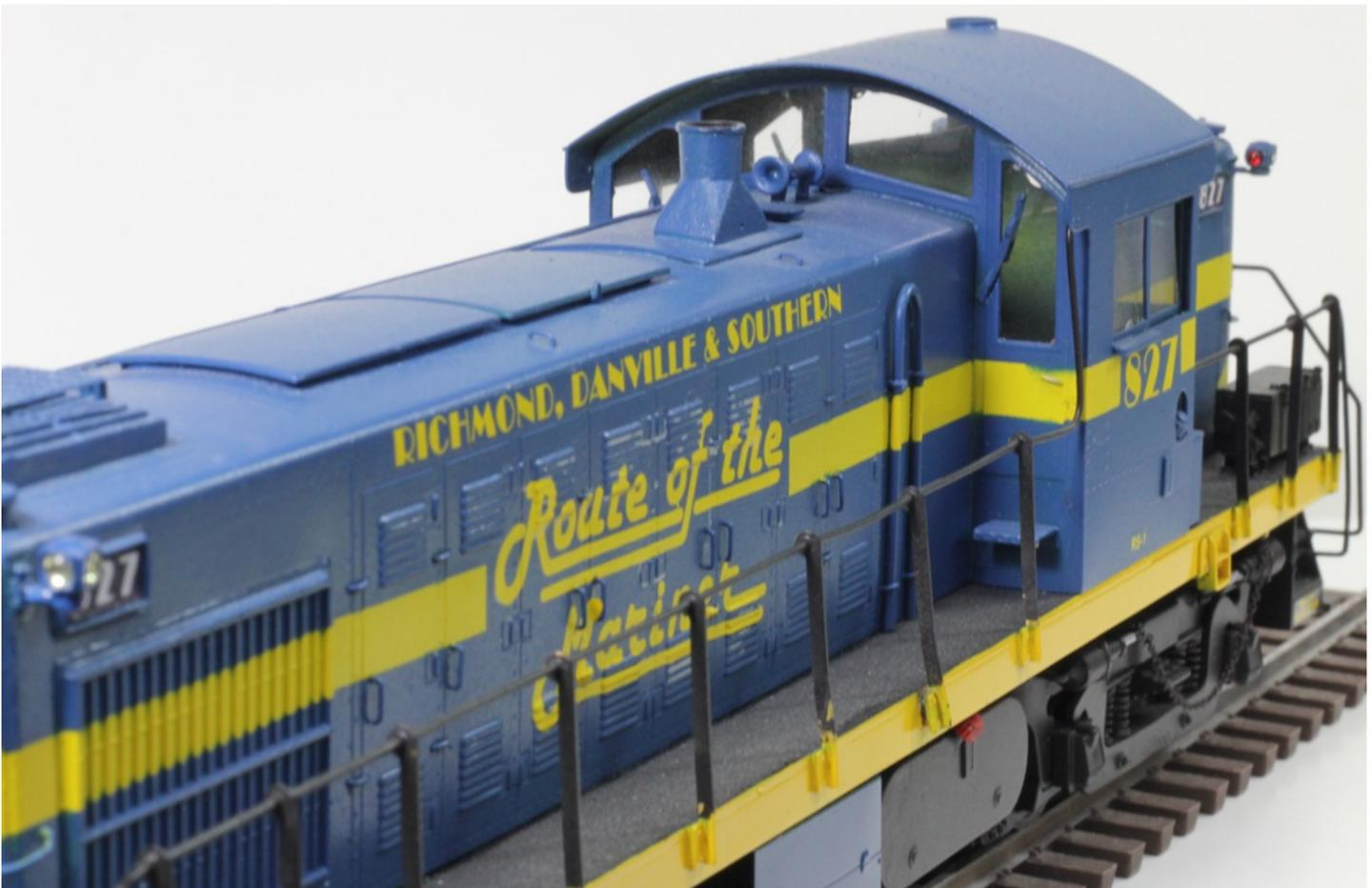
*This NJ International Alco RS-1 was a bit easier to cut the windshield for than the Atlas RS-1 shown in the video. Remember to leave room for the railings and wipers to pop though the shell. It's a mess if you forget.*
