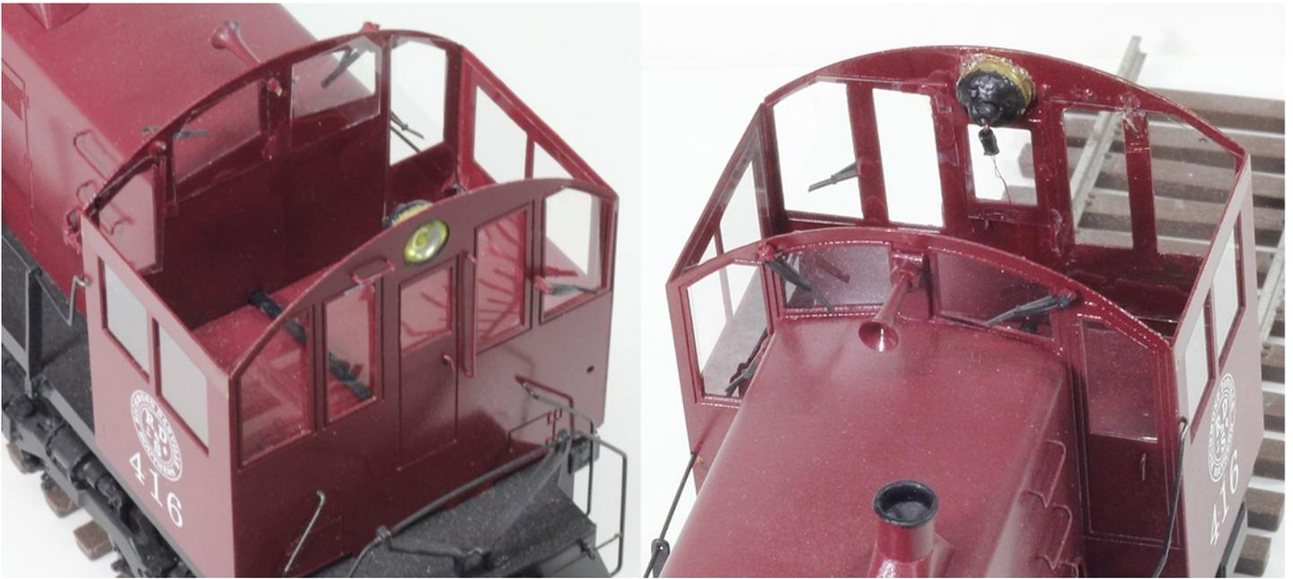
*Sometimes we can cheat and not have to cut curves. You can see some of the straight angles I was able to use in the cab of this Alco S2. This unit is begging for an interior which is in the works.*
