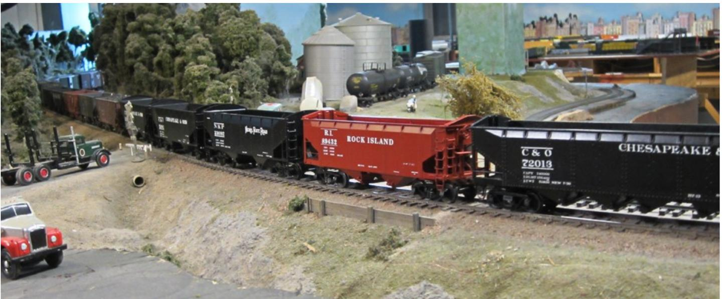
*C&O 4-bay and CRI&P 2-bay hoppers, both with trapezoidal heap shields lead a longer cut of coal hoppers, some with additional radial heap shields around a curve on the Des Plaines Valley layout mainline. The DPV layout was covered in the [August/ September 2014 issue of the S Scale Resource](#)*
