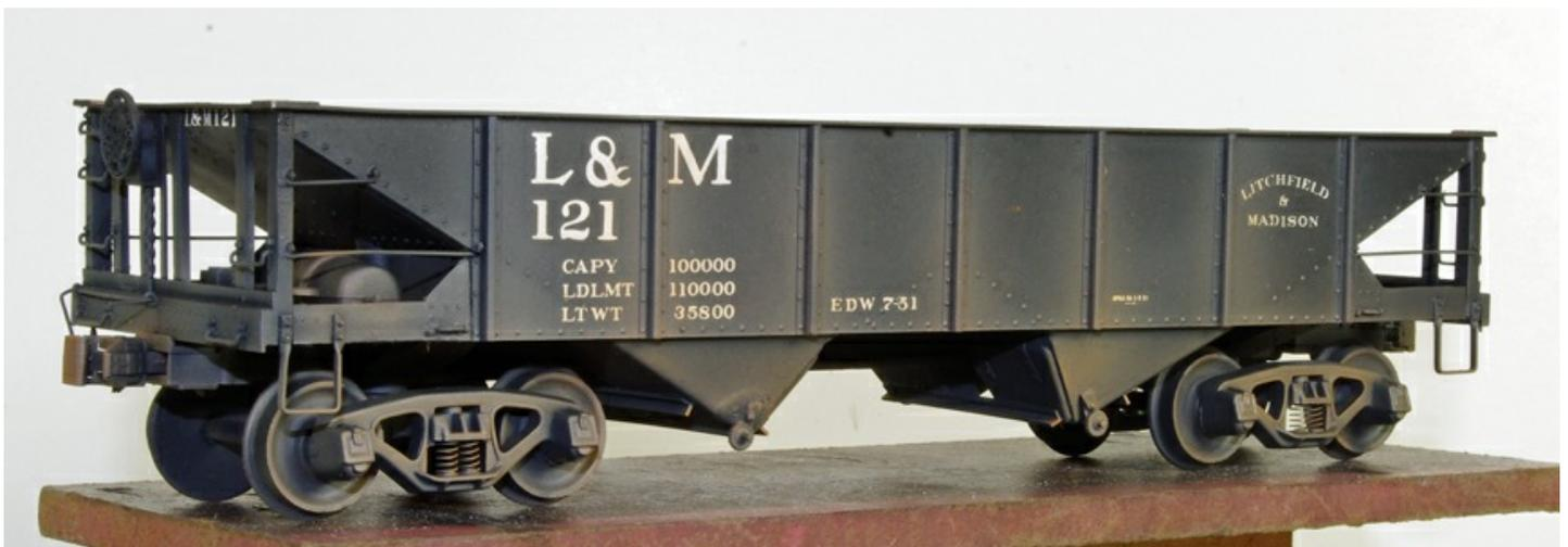
*Here is the side of the finished car. The dust was made with a very thin mix of rust and concrete color. Mix it up thin enough so you can't see it going on. It should look like you are just spraying clear thinner on the model. When the thinner evaporates, you will be left with dust.*
