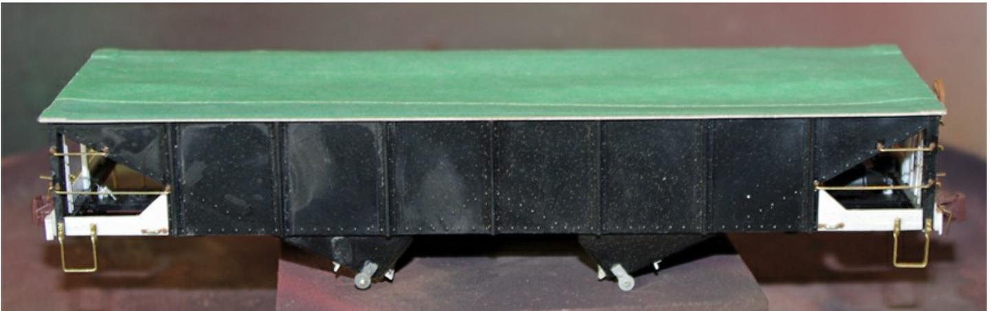
*I painted the interior of the car with a rust color first. Then, I masked a shown here so I could paint the exterior of the car.*
