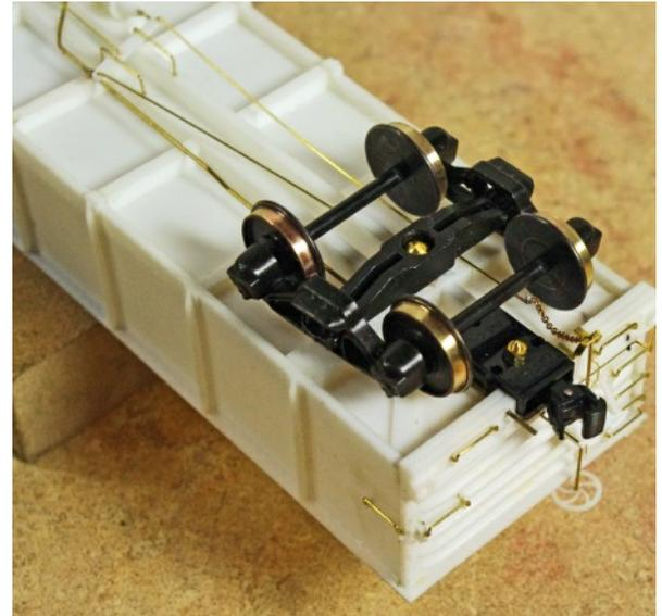
*On the left, you can see how the head of the flat head screw is flush with the floor and will hardly show when the car is painted. On the right, you can see the 0-80 nut holding the coupler on. Now I have a good solid mount that does not rely on threads into the resin.*
