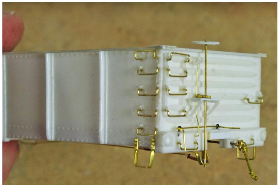
*These photos show some of the details on the car as I was going. Notice in the left photo how I located the center of the bolster for drilling. I used a brass threaded bushing to mount the coupler. This works better than threading the truck screw into the resin. Also, notice the 0-80 screw used to hold the coupler in place. I needed to add a piece of styrene to the end beam above the coupler – this is visible in the photo on the right.*
