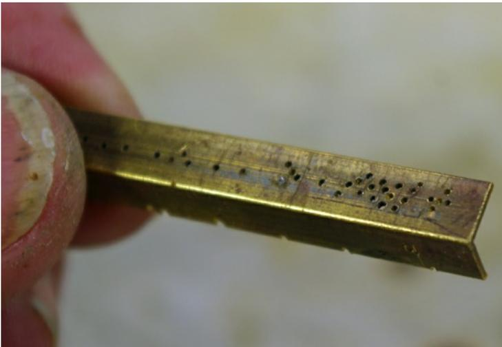
*I made this grab iron bending fixture from some scrap brass. You can see all the holes in it. I use it a lot. You can make this in styrene, but it will not hold up as well. A flat piece of brass will also work. I just happened to have this piece of angle, or I should say "it was the first thing I picked up".*
