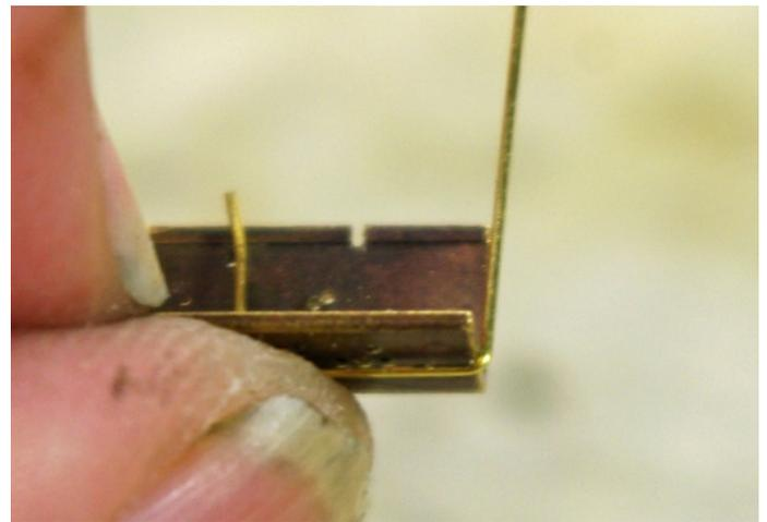
*To make a grab iron, bend one side first with some small pliers. Then, insert the piece into the correct hole on your fixture. Bend the end over with your fingers. Fix up the bends with the pliers and cut to length.*
