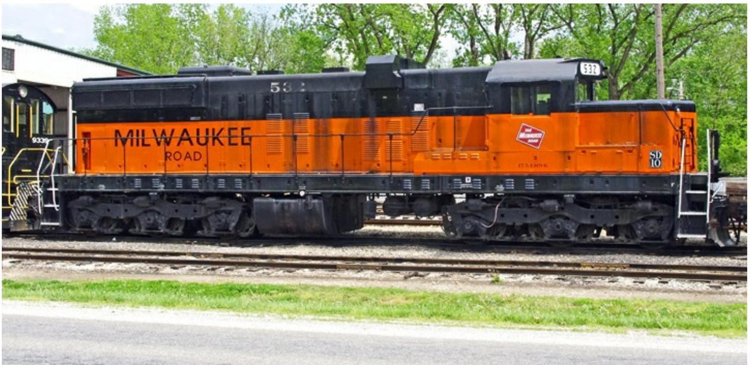
This Milwaukee SD-10 was photographed at the White Water Valley Railroad in Connersville, Indiana on the way home from the Spring S Spree in Dayton. The Milwaukee Road rebuilt SD-7's and SD-9's into SD-10's. The Milwaukee SD-7's were the first SD-7's, and some of the development work was done at Crivets, Wisconsin. The Milwaukee units were the lightest engines and had the small fuel tanks to keep weight down. This would be an interesting kit bash project.
