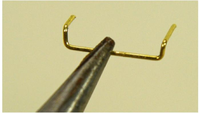
*To make a drop grab, hold the bent grab iron at the tip of some small pliers and bend it over as shown on the left. Remember where you held it in the pliers and do the same for the other side. If it helps, put a small mark with a Sharpie pen on the tip of the pliers so you know where to hold the grab iron. That way, they will all come out the same.*
