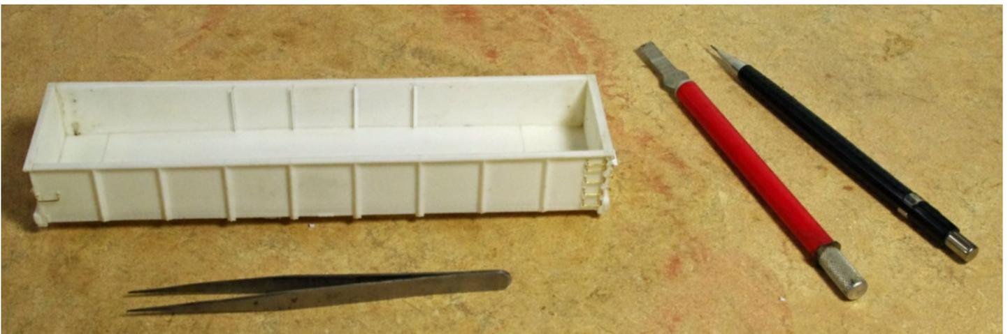
*Here are some of the tools I used to make the internal bracing. I like the chisel tip on the hobby knife better than the regular blade for cutting small pieces. The chisel blade has a flat side that gives a nice square cut. The fine line mechanical pencil is good for marking.*
