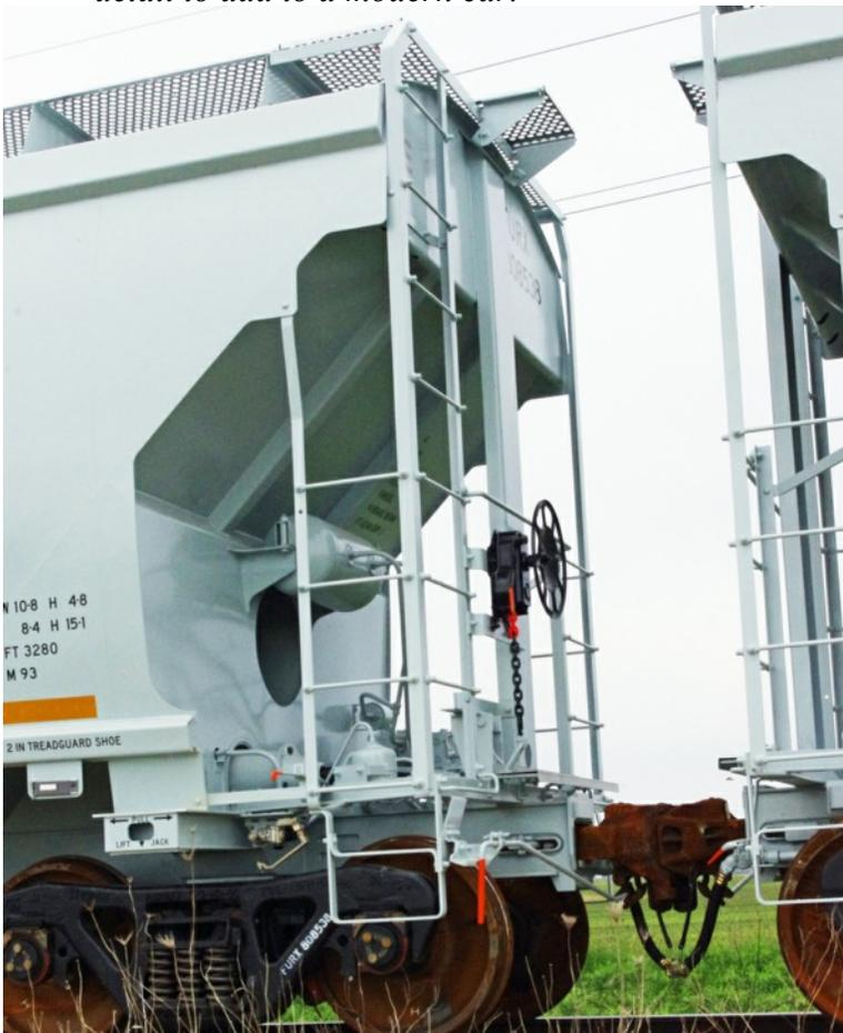
*Here are some details of the ends of the cars. Note that the brake wheel and gear box are painted black. This is another detail that could be done to a ready to run car.*
