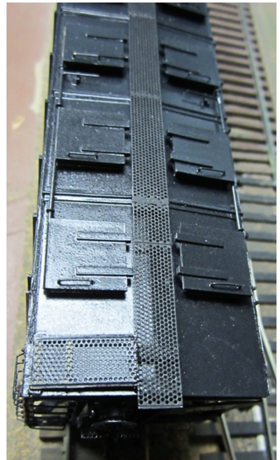
Photo 7: Here is the car with the Morton Roof Walk installed. I used short pieces of 0.010" x 0.040" styrene under the roof walk to help with mounting. The mounting points on the etching corresponded very well with the mounts cast in the resin covered hopper roof. One other tip - paint the roof walk assembly and roof separately and then attach the roof walk. Otherwise it is hard to paint the area under the roof walk without risking filling in many of the delicate holes in the high quality etching.
