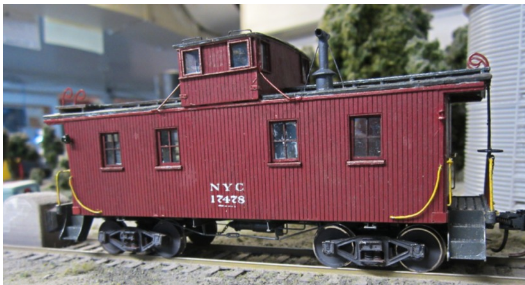
Photo 3: A side view of the finished caboose. The view shows the underbody turn buckle, truss rod and more K-brake details. Handrails and grab irons are all hand made. I used an old Floquil paint bottle as a form to bend the curved handrails on each of the caboose's four corners.
