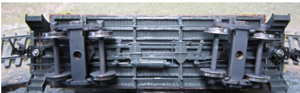
Photo 2: This is the brass frame attached to the caboose floor with trucks, K-brake and other underbody detail added. The level of brake detail is left up to the modeler. The underbody is painted a dark gray to simulate a more weathered appearance.
